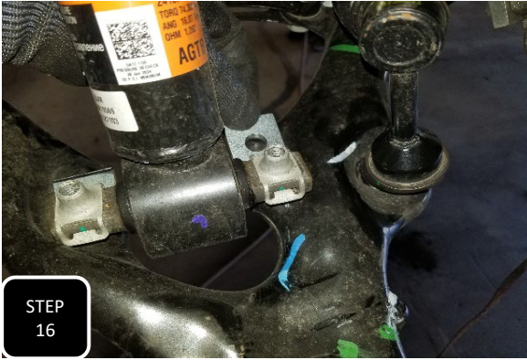
Step 16 Once both spacers are in place then re-install the factory bolts and tighten to 40 ft/lbs.
