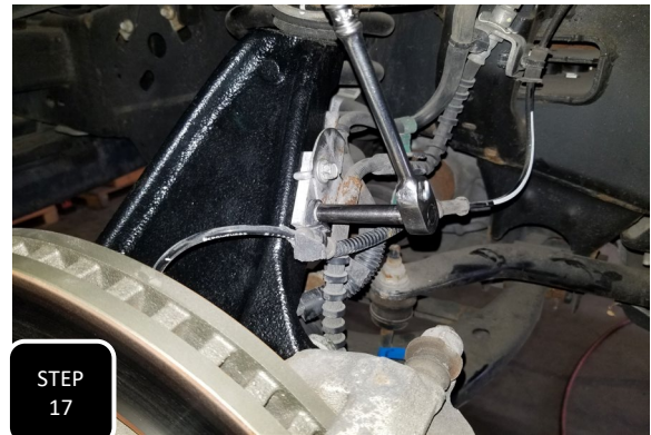
Step 17 Re-attach the brake line bracket and ABS line bracket to side of the spindle along with the provided spacer using the factory bolts. NOTE: THE GUIDE TAB ON THE BRAKE LINE BRACKET WILL NEED TO BE SLIGHTLY BENT TO CLEAR THE BRAKE LINE SPACER.
