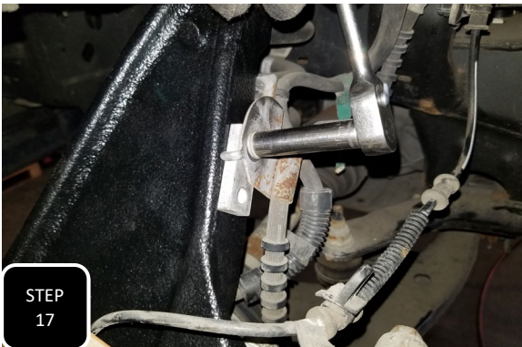
Step 17 Re-attach the brake line bracket and ABS line bracket to side of the spindle along with the provided spacer using the factory bolts. NOTE: THE GUIDE TAB ON THE BRAKE LINE BRACKET WILL NEED TO BE SLIGHTLY BENT TO CLEAR THE BRAKE LINE SPACER.
