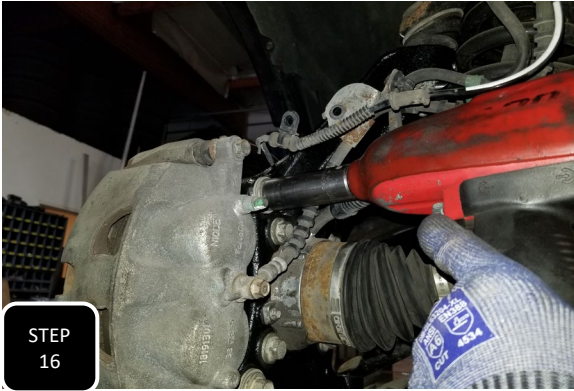
Step 16 Re-install the brake caliper using the factory bolts and tighten.
