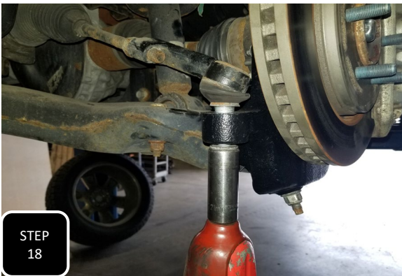
Step 18 Attach the tie rod to the steering arm on the spindle and tighten using the factory nut.
