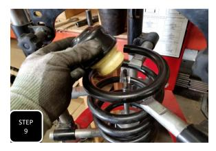
**Step 9** Slide the new coil seat onto the strut, then iinstall the strut up through the bottom of the coil. Next, slide then bump stop onto the shaft of the shock.
