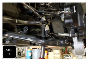
**Step 2** Unbolt and remove the sway bar end link.
