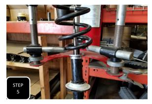
**Step 5** Once the nut is removed, pull the strut top off, remove the bump stop and remove the strut out the bottom of the coil.
