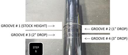
**Step 6** Locate your new struts and set the ring to the proper groove according to the chart above. Make sure the snap ring fully engages into the groove.
