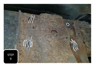
**Step 9** With the leaf springs now out of the way, you will need to remove the rear, shackle hanger by making multiple cuts into the head of each of the 3 mounting rivets using a 4.5" cut off wheel. The bolt at the upper hole can just be un-bolted and saved for re-installation.
