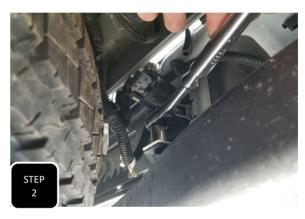
**Step 2** Unbolt the 6 bolts which attach the trailer hitch to the frame and remove the trailer hitch. **NOTE: THERE WILL** ALSO BE TWO SMALL BOLTS THAT ARE HIDDEN UP NEAR THE SPARE TIRE ATTACHING THE HITCH TO THE BUMPER.
