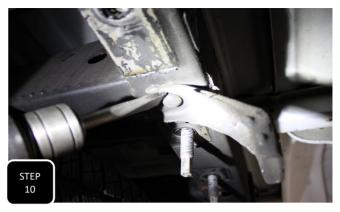
**Step 10** Next, you will need to chissel off the remainder of the heads using a pneumatic hammer with a chissel attachment and then finally punch out the body of the rivot using a pneumatic hammer with a punch attachment. Older models will have one more rivet attaching a support bracket to the bottom of the frame. This bracket will be welded on newer models and needs to be cut off.
