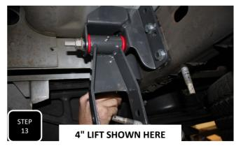
**Step 13** If installing the hangers in the 2 & 4 holes, you will need to bend the bed seem, directly above the spring hanger, for additional clearance.
