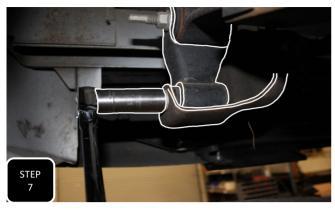
**Step 7** Unbolt the shackle mounting bolt on both sides and remove.
