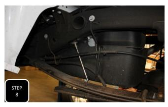
**Step 8** Working on one side at a time, remove the U-bolts and lower the axle away from the leaf spring. Next, pull the leaf spring/shackle out, around, and under the shackle mounting hanger. Now re-attach the leaf spring to the axle and torque the U-bolts to 100 ft/lbs. **REPEAT THIS STEP WITH THE OTHER LEAF SPRING.**
