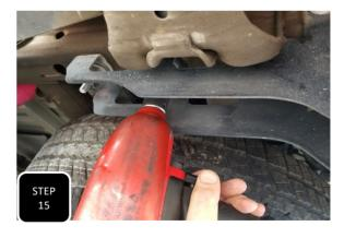
**Step 15** Jack the axle up and loosely attach the leaf spring to the shackle using the factory bolt facing from the inside, outward. Do not fully tighten any of the spring or shackle bolts until the truck is back on the ground at ride height. Next, re-install the trucks trailer hitch.
