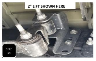
**Step 14** Attach the hanger with the shackle pre-assembled into it. The shackle can be installed with the open end facing either direction. The hanger will get attached using 3 of the provided 7/16" bolts and re-using the one factory bolt. **NOTE: THE SHACKLE CANNOT BE INSTALL AFTER THE HANGER IS INSTALLED.**
