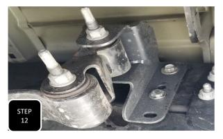
**Step 12** Before installing the hanger, attach the shackle to the hanger using the factory bolt, oriented from the inside out.
