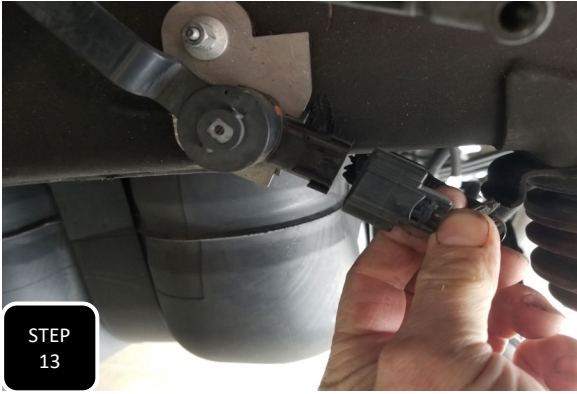
Step 13 Re-connect the plug at the sensor and then re-insert the red safety clip.
