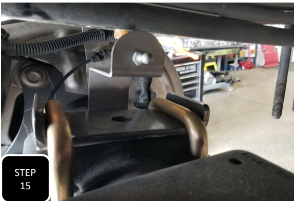
Step 15 For a 5" drop you will need to remove the mounting ball from the factory mounting plate and attach it to part # 3019MR-6, the taller of the two supplied mounting plates, using the supplied M6 flat washer and nut.
