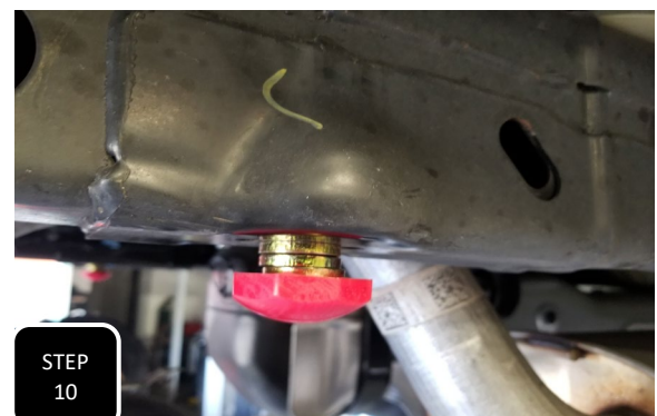
Step 9 The bed rib is made from a much thinner material and can be cleared using a hammer. NOTE: TO AVOID ANY CUTTING, YOU CAN ADD WASHERS TO SPACE THE BUMP STOPS DOWN, BUT THIS WILL EVEN FURTHER MINIMIZE YOUR LIMITED AMOUNT OF UPTRAVEL AND CAUSE FOR A ROUGHER RIDE.
