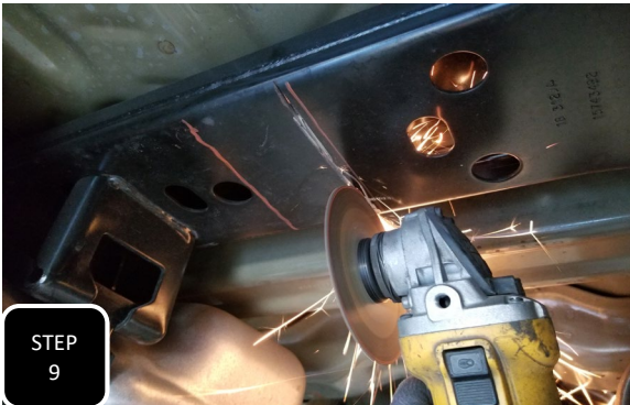
Step 9 Using an angle grinder with a cut off wheel, cut the cross member on your marked lines and then at each end to connect the lines. Next, remove the piece that was cut out, clean up any sharp edges, and spray paint for rust prevention. NOTE: YOU ARE ONLY REMOVING THE THICKNESS OF THE BOTTOM OF THE CROSSMEMBER. THE THREE DIMENSIONAL STRENGTH OF THE CROSS MEMBER IS STILL INTACT.
