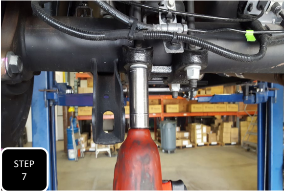
Step 7 Unbolt the U-bolts, on the driver's side only and remove the U-bolts.
