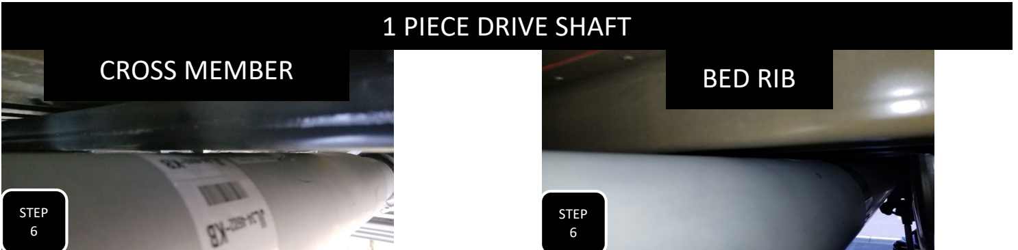
Step 6 Models with a 1 piece drive shaft have a cross member and a bed rib, both located closer to the transmission, that the drive shaft will slightly contact when the suspension bottoms out.
