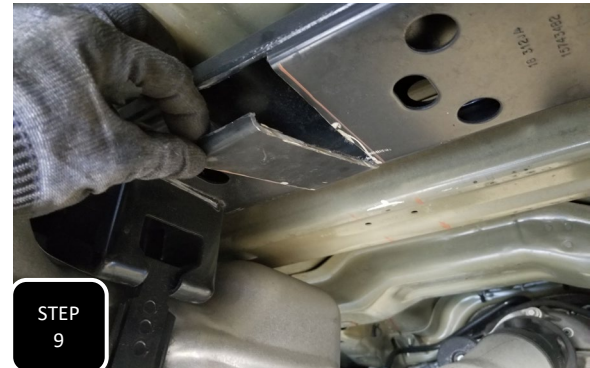
Step 9 Using an angle grinder with a cut off wheel, cut the cross member on your marked lines and then at each end to connect the lines. Next, remove the piece that was cut out, clean up any sharp edges, and spray paint for rust prevention. NOTE: YOU ARE ONLY REMOVING THE THICKNESS OF THE BOTTOM OF THE CROSSMEMBER. THE THREE DIMENSIONAL STRENGTH OF THE CROSS MEMBER IS STILL INTACT.
