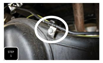
**Step 1** The hard brake lines on the axle housing have guide clamps that orient downward. Unbolt the clamps, remove and re-install them facing upward.
