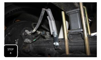
**Step 4** Moving to the front of the axle, locate the two E-brake cable brackets located just outward of the leaf spring mounts. Unbolt the guide brackets and install the new E-brake extension brackets with the bent side facing up and attach using the provided M8 hardware at the brackets and the factory bolt at the axle.
