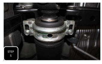
**Step 5** Locate the carrier bearing in the middle of the two drive shafts and loosen, but do not fully remove both bolts.
