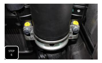
Step 6 One at a time, remove a carrier bearing mounting bolt and install one of the provided spacers along with the new M10 bolt and washers. The spacer will have a yellow sticker with an arrow on it. This sticker needs to face the front of the truck with the arrows pointed upward. This will give the carrier bearing a little bit of a downward slope towards the axle.
