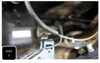
**Step 3** Locate the ABS line guide bracket on the axle (Driver's side), open up the clamp and remove the ABS wire. **NOTE: THIS ALLOWS FOR MORE SLACK WHILE THE AXLE IS AT FULL DROOP.**
