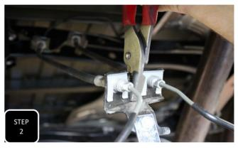
**Step 2** Unbolt the brake line bracket at the top of the differential, gently stretch the harlines to space the bracket up from the diff, and then install the new brake line bracket using the provided M8 hardware at where the brackets meet and the factory bolt at the diff.
