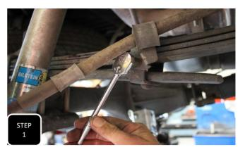
**Step 1** Unbolt the E-brake cable from the frame and the outside of the leaf spring on both sides of the truck.
