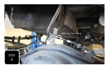
**Step 8** Cut the zip tie attaching the ABS line to the bracket on top of the differential, then loosen the mounting bolt for the bracket and rotate the bracket vertical and tighten.
