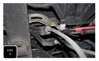
**Step 4** Locate the brake line bracket on the frame and slightly bend the mounting tabs downward so that the end of the line points at the other end.
