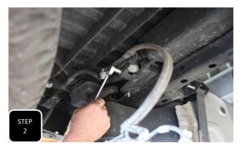
**Step 2** Unbolt the ABS line from the top of the differential and at the frame.
