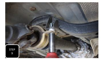
Step 9 Loosen both bolts attaching the carrier bearing to the frame, but do not remove. One at a time, remove one bolt, install a spacer between the carrier bearing and frame, then attach using the provided M10 bolt and washers. Next, install the other side and torque both bolts to 30 ft/lbs.
