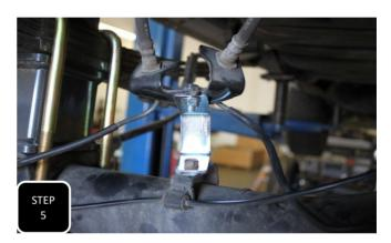
**Step 5** Unbolt the brake line bracket from the top of the axle housing, gently stretch the hardlines to gain slack between the axle and bracket, then install the new brake line bracket using the factory bolt at the axle and the provided M8 hardware where the brackets meet.
