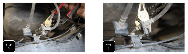
**Step 3** Locate the brake line bracket on the axle housing. Using a pair of channel locks or a cresent wrench, bend the two brake line connection tabs back so that the soft line end points up at itself. **NOTE: BENDING THIS BRACKET CREATES MORE SLACK IN THE SOFT LINE.**
