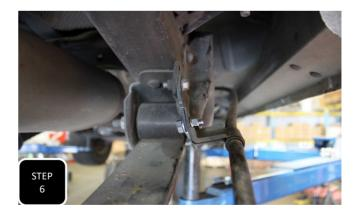
Step 6 Locate the provided E-brake brackets with the notch in the side and install them at the frame E-brake mount with the notch facing the rear of the truck and the bend pointing outward. Attach them to the frame using the factory bolt and to the E-brake cable using the provided M8 hardware.
