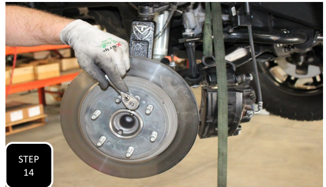
Step 14 Slide the rotor onto the wheel studs and attach it to the hub using the factory retainer bolt.
