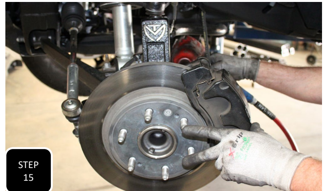
Step 15 Remove the clip that attaches the soft brake line to the frame and pull the hard line through the bracket to gain slack in the line. Next, install the brake caliper using the factory bolts and tighten to factory specs.
