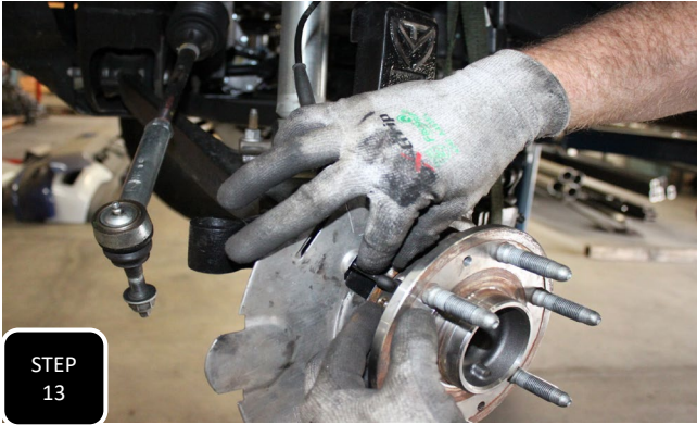
Step 13 Install the ABS sensor and attach it using the factory bolt.
