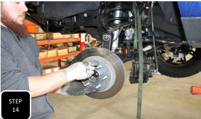
Step 14 Slide the rotor onto the wheel studs and attach it to the hub using the factory retainer bolt.
