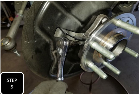
Step 5 Unbolt the ABS sensor from the wheel bearing and also unbolt the wire guide bracket on the back side of the spindle. Hang the sensor out of the way so that it does not get damaged during the install.
