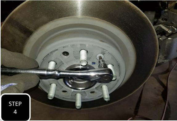
Step 4 Unbolt the retainer screw attaching the rotor to the drive flange and remove the rotor.
