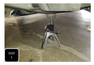
**Step 1** Jack up the front of the of the vehicle and support under the frame rails with jack stands. Remove both front tires and proceed with one side at a time.
