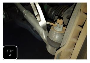
**Step 2** Remove the cotter pin that is engaged in the outer tie rod end.
