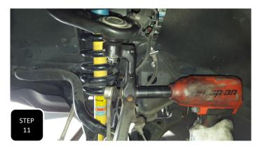
**Step 11** Re-attach the sway bar end link to the spindle and tighten. **NOTE: THIS STEP SHOULD BE DONE AFTER THE SPACERS HAVE BEEN INSTALLED ON BOTH SIDES.**
