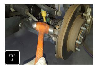
**Step 3** Loosen the tie rod nut, then break the tie rod loose by hitting the side of the steering arm with a hammer and separate. **NOTE: NEVER HIT THE TIE ROD ON THE THREADS.**
