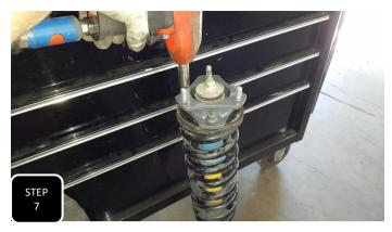
**Step 7** Remove the strut and then attach the strut spacer to the top of the strut using the factory nuts and tighten.
