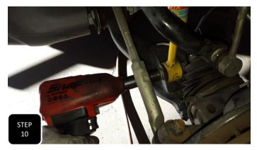
**Step 10** Tighten the provided nuts at the top of the strut and the factory bolt at the bottom.
