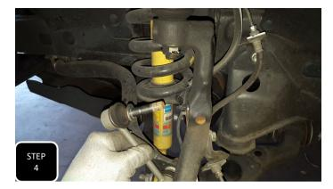
**Step 4** Unbolt the sway bar end link from the neck of the spindle and separate.
