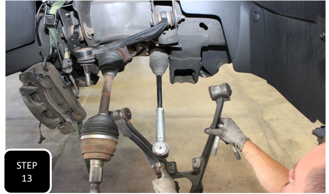
Step 13 Unbolt both lower control arm mounting bolts and remove the lower control arm.
