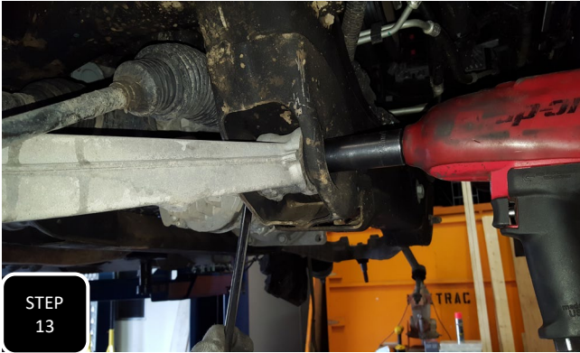
Step 13 Unbolt both lower control arm mounting bolts and remove the lower control arm.
