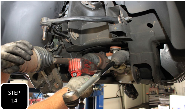
Step 14 Unbolt all 6 bolts attaching the CV axle to the differential housing and remove the axle.
