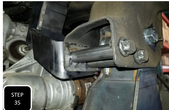
Step 35 Locate the passenger side diff drop support bracket and loosely install it between the passenger side diff bracket and the frame where the rear cross member was original located. Install the provided sleeves in the gap of the frame and use the factory bolts through the sleeves and into the support bracket. Once all are loosely installed, fully tighten all 3 bolts to 85 ft/lbs.
