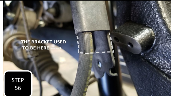
Step 56 Attach the brake line guide bracket to the side of the spindle using the factory M6 bolt and tighten. Next, pull the brake line down through the mounting bracket to gain some slack between the brake caliper and mounting bracket.
