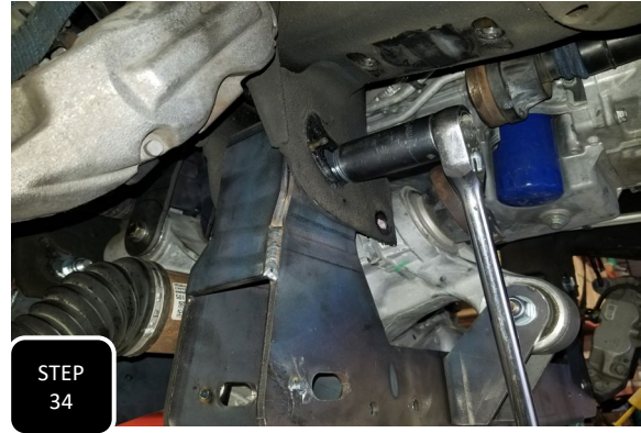
Step 34 Fully tighten all 4 bolts that attach the subframes to the frame and torque to 170 ft/lbs.
