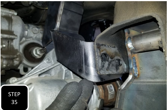
Step 35 Locate the passenger side diff drop support bracket and loosely install it between the passenger side diff bracket and the frame where the rear cross member was original located. Install the provided sleeves in the gap of the frame and use the factory bolts through the sleeves and into the support bracket. Once all are loosely installed, fully tighten all 3 bolts to 85 ft/lbs.
