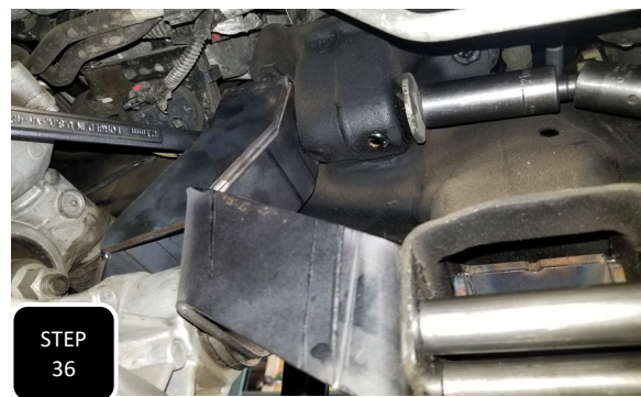
Step 36 Fully tighten the passenger side diff drop bracket to the frame and torque to 85 ft/lbs.
