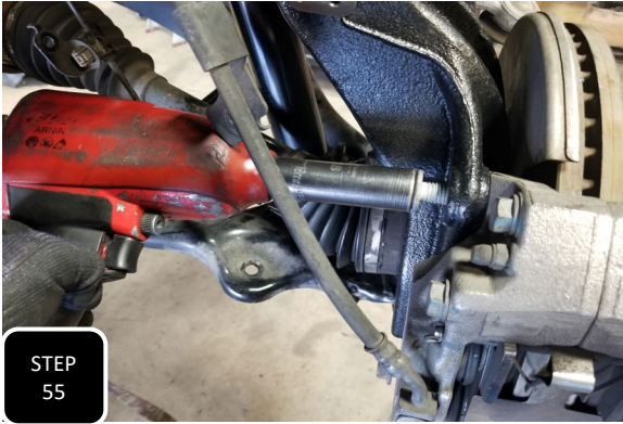
Step 55 Install the brake caliper using the factory bolts and torque to factory specs.
