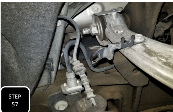
Step 57 Unclip the ABS line from the mounting bracket at the upper control arm to gain slack in the line. Next, install the ABS sensor in the mounting hole at the front of the steering knuckle and attach it using the factory M6 bolt.
