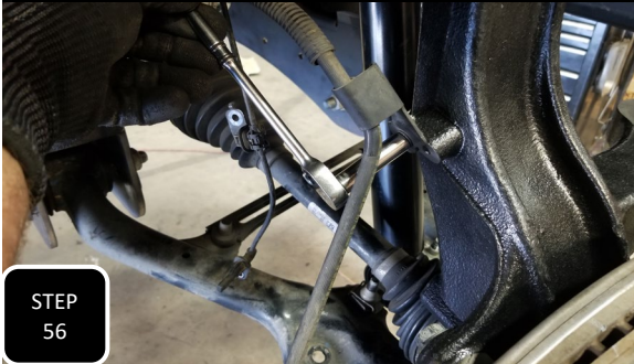
Step 56 Attach the brake line guide bracket to the side of the spindle using the factory M6 bolt and tighten. Next, pull the brake line down through the mounting bracket to gain some slack between the brake caliper and mounting bracket.
