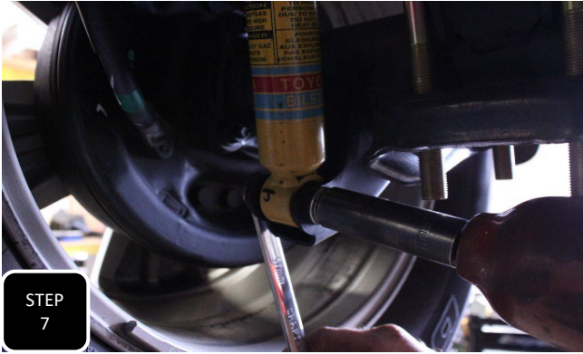
Step 7 Unbolt both rear shocks at both ends and remove.
