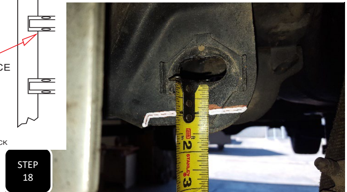
Step 18 Measure 3/4" down from the forward facing hole of the rearward lower control arm mounts and mark a line all the way across the bracket, parallel to the slotted hole.
