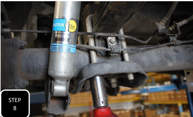
Step 8 Working on one side at a time, unbolt the U-bolts and remove them along with the lower spring plate.
