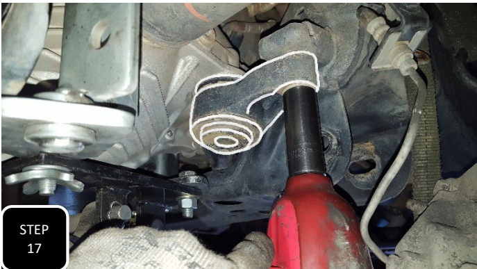
Step 17 Unbolt both mounting bolts for the driver's side rear diff mount and then remove the mount.
