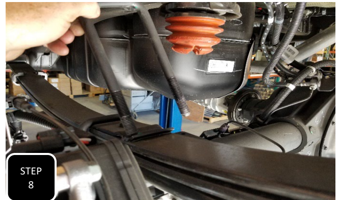
Step 8 Working on one side at a time, unbolt the U-bolts and remove them along with the lower spring plate.
