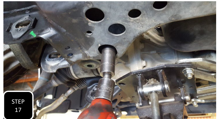
Step 17 Unbolt both mounting bolts for the driver's side rear diff mount and then remove the mount.
