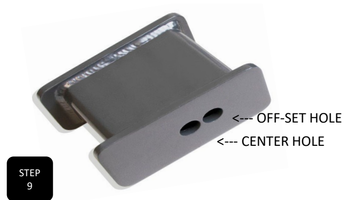
Step 9 Lower the axle down enough to make room for the new lift block and install the new lift block. The short end of the block will face the front of the truck and the tall end will face the rear of the truck. The lift block features two center pin holes, you will line up the leaf spring center pin with the offset hole in the block, which will push the axle 1" forward. NOTE: IT WILL HELP TO SLIGHTLY LOOSEN THE U-BOLTS ON THE OTHER SIDE, BUT DO NOT FULLY LOOSEN THEM.
