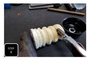
**Step 8** Locate the factory bump stop, remove it from the metal cup, and cut one rib off of the end of it.
