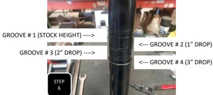
**Step 6** Locate your new struts and set the ring to the proper groove according to the picture above. Make sure the snap ring fully engages into the groove.
