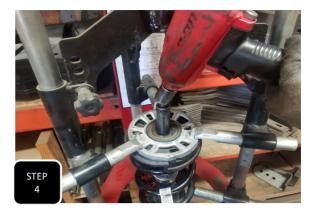
**Step 4** Using an automotive coil/strut compressor, compress the coil so that the strut can be disassembled safely and then remove the nut at the center of the strut top. **NOTE: TAKE NOTE OF THE RELATIONSHIP BETWEEN THE STRUT TOP AND THE STRUT BOTTOM FOR PROPER CLOCKING DURING INSTALLATION.**
