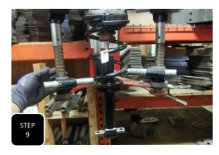
**Step 9** Slide the new coil seat onto the strut, then install the strut up through the bottom of the coil. **NOTE: MAKE SURE TO INSTALL THE BUMP STOP UP INTO THE CUP ON THE BOTTOM OF THE STRUT TOP BEFORE INSTALLING THE STRUT.**
