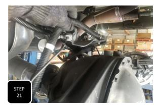
**Step 21** Unbolt the three bolts attaching the brake line bracket to the top of the differencial then pull it slightly up and forward.
