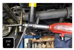
**Step 26** Install the new shorter shocks with the shaft of the shock attached at the frame and the body of the shock attached at the axle. **NOTE: IF YOU PURCHASED SHOCK EXTENDERS, NOW WOULD BE THE TIME TO INSTALL THEM ALONG WITH THE FACTORY SHOCKS. USE THE EXTENDER INSTRUCTIONS FOR INSTALL.**
