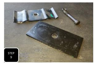
**Step 9** The leaf pack will now need to be dis-assembled. Attach two clamps to the spring and remove the center pin along with the U-bolt retainer plate and the factory 2 degree shim. (Only 2019 models have this shim) **NOTE: DISCARD THE U-BOLT RETAINER PLATE. IT DOES NOT GET RE-USED.**
