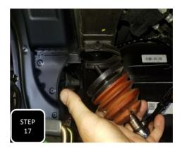
**Step 17** Unbolt both of the factory rear bump stops from the frame and remove.
