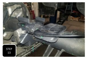
**Step 13** For 2020-2023 models, place the supplied 2 degree shim on the center pin with the thick end facing the rear of the truck. For 2024+ models, place the shim with the thick end facing the front of the truck. Next, place the axle relocator on top of the shim with the brake line mounting bracket facing rearward. Slightly loosen the U-bolts on the other side and then lower the axle into the relocator.
