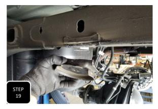
**Step 19** Once both cuts are made, it may help to hit the cut piece with a hammer until it breaks loose and then remove it from the frame. Next, clean up any sharp edges and spray paint for rust prevention.
