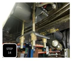
**Step 14** Place the U-bolt retainer plate on top of the original spring plate and run the new U-bolts downward though the provided spring perch under the leaf pack and tighten. **NOTE: THE U-BOLTS WILL INSTALL JUST LIKE THE FACTORY ONES DID. DO NOT TORQUE THE U-BOLTS DOWN AT THIS TIME.**
