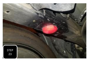
**Step 23** Insert the bump stop nut plates into the hole in the bottom of the frame that emerged after you removed the driver's and passenger's side factory bump stop plate. Thread the provided low profile bump stop into the nut plate until tight.
