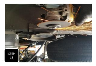
**Step 18** Unbolt the brake line guide bracket on the inside of the driver's side frame rail and support out of the way. Next, you will need to cut off the welded on bump stop plate using a suitable cutting device. Make a clean cut on each side of the frame rail.
