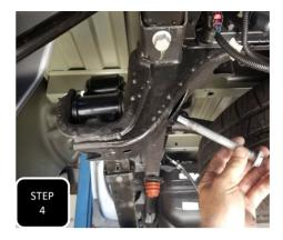
**Step 4** Loosen then remove the bolt attaching the shackle to the frame.
