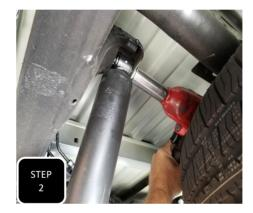
**Step 2** Jack up the adjustable jack slightly to apply pressure to the axle then unbolt both shocks at both ends and remove.
