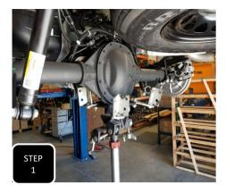
**Step 1** Jack up the rear of the vehicle and support under the frame rails with jack stands. Leave an adjustable jack under the differencial for height adjustment.
