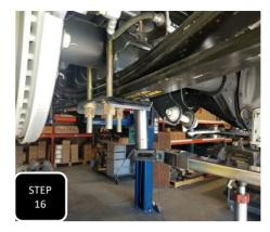
**Step 16** Repeat steps 3-13 on the other side then when both sides are complete, torque the U-bolts to 100 ft/lbs.
