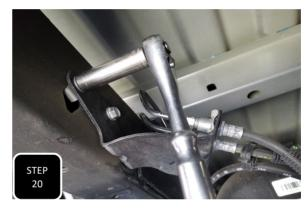
**Step 20** Once spray painted, re-install the brake line bracket using the factory bolts and tighten.
