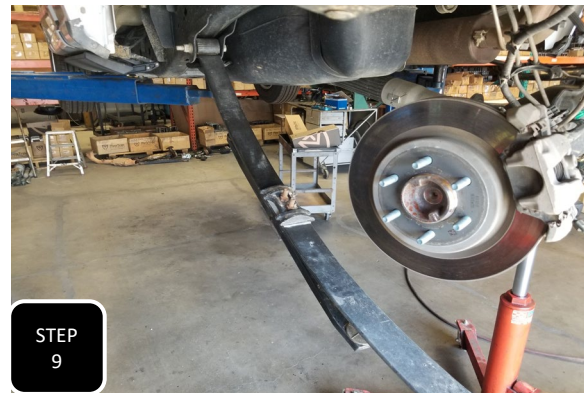
Step 9 Double check that the axle is balanced & properly secured to an adjustable jack on wheels. Lower the axle and roll it towards the passenger side. Next, lower the leaf spring around the axle and then re-center the axle under the truck. NOTE: BE CAUTIOUS NOT TO OVER EXTEND ANY WIRES OR BRAKE LINES
