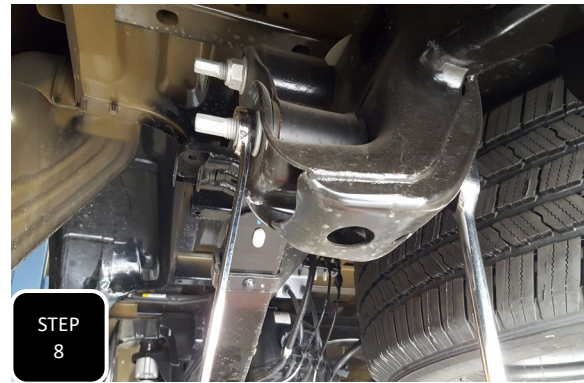
Step 8 Working on only the driver's side, loosen the bolt at the front of the leaf spring and then unbolt the shackle from the frame. Next, remove the shackle bolt at the frame.
