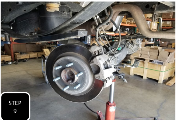
Step 9 Double check that the axle is balanced & properly secured to an adjustable jack on wheels. Lower the axle and roll it towards the passenger side. Next, lower the leaf spring around the axle and then re-center the axle under the truck. NOTE: BE CAUTIOUS NOT TO OVER EXTEND ANY WIRES OR BRAKE LINES
