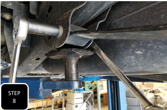
Step 8 Working on only the driver's side, loosen the bolt at the front of the leaf spring and then unbolt the shackle from the frame. Next, remove the shackle bolt at the frame.
