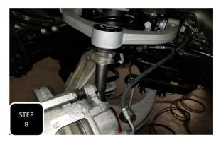
**Step 8** Attach the upper control arm to the spindle using the provided nylock nut and washer, then tighten.
