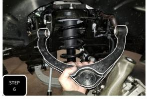
**Step 6** Pull the upper ball joint out of the spindle and gently allow the spindle to flop to the side. Next, remove the upper control arm.
