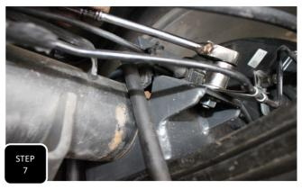
**Step 7** Jack up the rear axle and support under the frame with jack stands. Working on one side at a time, remove the U-bolts then unbolt the brake line guide bracket from the axle relocator.
