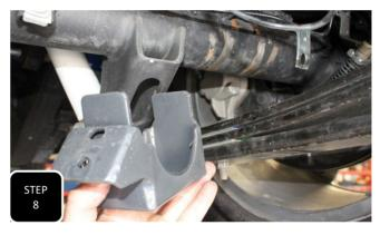
**Step 8** Jack the axle up off of the leaf pack and remove the axle relocator.
