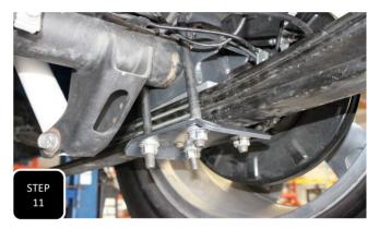
**Step 11** Re-install the axle relocator, lower the axle into it and loosely install the U-bolts. Next, re-attach the brake line guide bracket to the relocator. **NOTE: DO NOT FULLY TIGHTEN THE U-BOLTS UNTIL BOTH SHIMS HAVE BEEN INSTALLED.**
