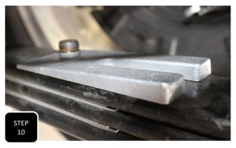
**Step 10** Remove the clamps and install the provided 4 degree shim with the center pin in the round hole and the thick end facing the rear of the truck.
