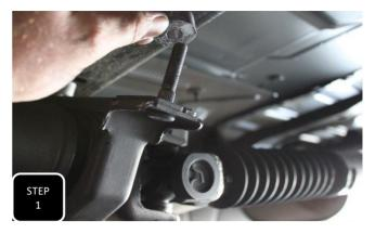
**Step 1** Unbolt the carrier bearing from the cross member and support with a strap or bungy cord. Next, remove the factory, 1/2" spacers and save for re-installation. **NOTE: THE SPACERS WILL BE A LITTLE BIT TOUGH TO REMOVE BECAUSE THE NURLING OF MOUNTING STUDS PRESS INTO THEM.**
