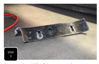
**Step 3** Using a suitable cutting device, cut through your lines and remove the middle of the cross member.
