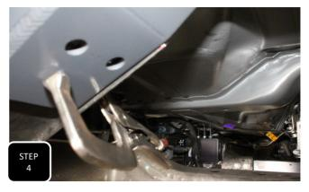
**Step 4** Push the new, MaxTrac cross member up tight against the remainder of the factory cross member with the vertical side facing the rear of the truck. Loosely install two of the supplied bolts through the holes on the vertical side of the cross member and then sinch down the cross member using clamps.
