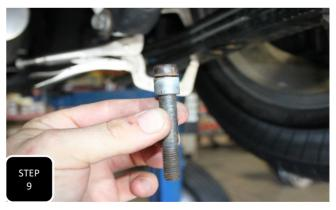
**Step 9** Place two clamps on the leaf pack to hold it together and then remove the center pin. Next, install the provided sleeve onto the center pin and then re-install it the same way it came off.
