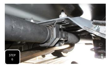
**Step 6** Attach the carrier bearing to the new cross member using the factory nuts and the factory 1/2" spacers, now installed on top of the cross member and tighten.
