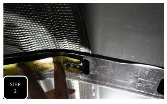
**Step 2** Hook a tape measure on the original carrier bearing mounting slotted hole, measure 3" away and mark a line a line across the bottom of the cross member. Next, repeat on the other mounting hole.
