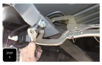
**Step 5** Using the MaxTrac cross member as a guide, drill 4 new holes up into the factory cross member and loosely install the provided 7/16" hardware. Once all 4 holes are drilled, tighten down all 6 bolts and torque to 40 ft/lbs.
