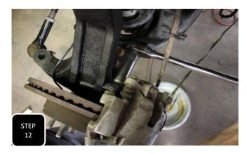
**Step 12** Attach the brake caliper to the spindle using the factory bolts and torque to 80 ft/lbs.
