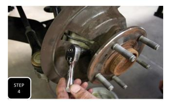
**Step 4** Remove the rotor and place it off to the side. Next, unbolt the ABS sensor and swing it safely out of the way so it does not get damaged during the install.
