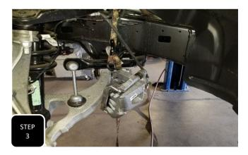
**Step 3** Unbolt the brake caliper and support out of the way with a strap. **NOTE: NEVER ALLOW THE CALIPER TO HANG FROM THE BRAKE LINE.**
