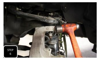
**Step 6** Loosen the upper ball joint nut, but do not remove. Next, break the ball joint loose by hitting the side of the spindle, right at the ball joint, with a hammer. The nut will catch the spindle then remove the nut. **NOTE: NEVER HIT THE BALL JOINT ON THE THREADS.**
