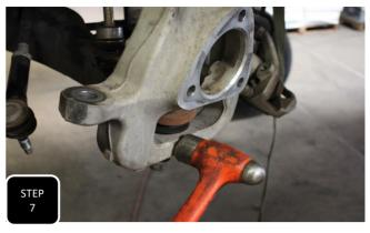
**Step 7** Loosen the lower ball joint nut, but do not remove. Next, break the ball joint loose by hitting the side of the spindle, right at the ball joint, with a hammer. The nut will catch the spindle then remove both the nut and the spindle. **NOTE: NEVER HIT THE BALL JOINT ON THE THREADS.**
