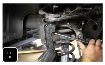
**Step 8** Locate the new spindle that matches the orientation of the spindle that you just removed and install it. The lower ball joint will get torqued to 150 ft/lbs. The upper ball joint has limited access and will get tightened down using a 12 point, 21mm combination wrench. **NOTE: IF THE UPPER BALL JOINT SPINS WHEN TIGHTENING, USE A PRY BAR ON TOP OF THE UPPER CONTROL ARM TO WEDGE THE BALL JOINT INTO THE TAPERED HOLE WHILE TIGHTENING.**
