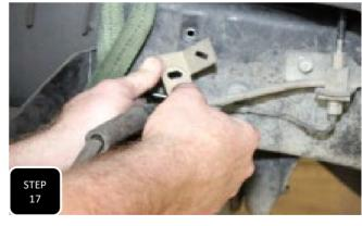
**Step 17** Starting with the driver's side, unbolt the mounting bracket closest to the soft line. Next, gentely bend the hard line downward and outward to make room for the new bracket. Lastly, slightly unravel the mounting bracket on the hardline so that it is at about a 30 degree angle.
