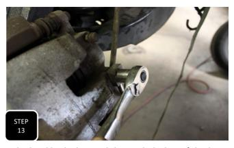
**Step 13** Using a line wrench, break loose the soft brake line from the hard brake line and then unbolt the soft brake line from the brake caliper.
