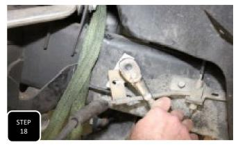
**Step 18** Attach the new brake line bracket to the frame using the factory bolt and then to the bracket on the stock hardline using the provided 1/4" hardware and tighten.
