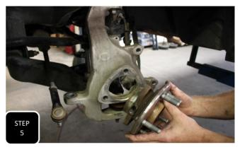
Step 5 Unbolt the 3 wheel bearing mounting bolts and remove the hub assembly. **NOTE: THE FACTORY DUST SHIELD WILL NOT GET RE-INSTALLED.**
