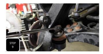
**Step 9** Install the wheel bearing "without" the factory dust shield. You will use two of the provided M14 bolts for the lower two mounting bolts and one factory mounting bolt for the top mounting bolt. All 3 bolts will get torqued to 120 ft/lbs.
