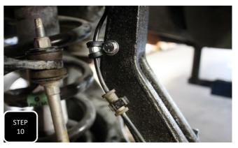
**Step 10** Install the ABS sensor using the factory allen bolt. Next, route the ABS line up the neck of the spindle and attach it to the neck of the spindle at one point with the factory plastic clip, and just above that with the provided 1/4" Adel clamp and provided M6 bolt.
