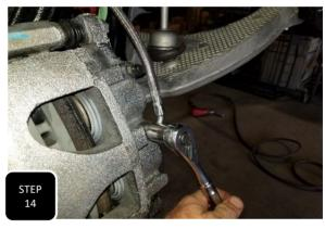
**Step 14** Attach the new, extended brake line to the hard line at the frame first and allow fluid to run through the line before attaching it to the brake caliper. Next, attach the brake line to the brake caliper using the factory banjo bolt and the provided copper crush washers. **NOTE: THE BRAKE LINE SHOULD BE POINTED STAIGHT UP FROM THE CALIPER.**
