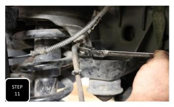
**Step 11** Slide the brake rotor onto the wheel bearing. Next, unbolt the brake line at the frame and slightly stretch the factory harline so it is easier to access the hardline to soft line connection.
