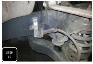
**Step 19** The passenger side is much simpler and only requires unbolting, pulling the hard brake line down, and then attaching the provided bracket. If you would like, the provided brake lines, although intended for the 2006-2022 models, will fit on the this side of the truck.
