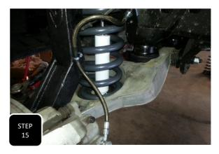
**Step 15** Push the end of the soft line up against the frame and attach using the provided "U" shaped clip and tap it into place using a hammer. Next, attach the brake line to the neck of the spindle using the supplied 3/8" Adell clamp and M6 bolt. **NOTE: YOU WANT THE LINE TIGHT FROM THE CALIPER TO THE CLAMP TO CREATE AS MUCH SLACK AS POSSIBLE BETWEEN THE CLAMP AND FRAME MOUNT.**
