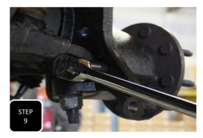
**Step 9** Install the wheel bearing "without" the factory dust shield. You will use the provided M14 bolt for the upper mounting bolt and two factory mounting bolts for the lower mounting bolts. All 3 bolts will get torqued to 120 ft/lbs.
