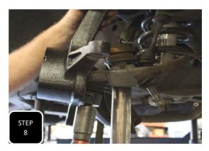
**Step 8** Locate the new spindle that matches the orientation of the spindle that you just removed and install it. The lower ball joint will get torqued to 150 ft/lbs. The upper ball joint will get torqued to 100 ft/lbs. **NOTE: IF THE UPPER BALL JOINT SPINS WHEN TIGHTENING, USE A PRY BAR ON TOP OF THE UPPER CONTROL ARM TO WEDGE THE BALL JOINT INTO THE TAPERED HOLE WHILE TIGHTENING.**
