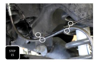
**Step 15** Push the end of the soft line up against the frame and attach using the provided "U" shaped clip and tap it into place using a hammer. Next, attach the brake line to the ABS line using two of the attached 3" zip ties. **NOTE: THE BRAKE LINE SHOULD BE ROUTED IN GRADUAL, SWOOPING FASHION AND BE SURE THAT IT DOES NOT CONTACT THE TIRE.**
