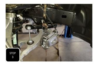
**Step 3** Unbolt the brake caliper and support out of the way with a strap. **NOTE: NEVER ALLOW THE CALIPER TO HANG FROM THE BRAKE LINE.**
