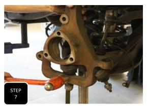
**Step 7** Loosen the lower ball joint nut, but do not remove. Next, break the ball joint loose by hitting the side of the spindle, right at the ball joint, with a hammer. The nut will catch the spindle then remove both the nut and the spindle. **NOTE: NEVER HIT THE BALL JOINT ON THE THREADS.**
