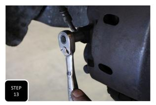
**Step 13** Using a line wrench, break loose the soft brake line from the hard brake line and then unbolt the soft brake line from the brake caliper.
