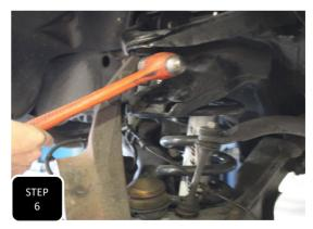
**Step 6** Loosen the upper ball joint nut, but do not remove. Next, break the ball joint loose by hitting the side of the spindle, right at the ball joint, with a hammer. The nut will catch the spindle then remove the nut. **NOTE: NEVER HIT THE BALL JOINT ON THE THREADS.**
