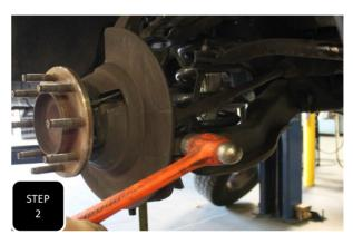
**Step 2** Unbolt the nut at the tie rod and break it loose by hitting the spindle with a hammer, right at the tie rod. **NOTE: NEVER HIT THE TIE ROD ON THE THREADS.**
