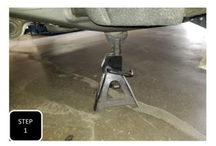
**Step 1** Jack up the front of the of the vehicle and support under the frame rails with jack stands. Remove both front tires and proceed with one side at a time.
