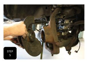
**Step 5** Unbolt the 3 wheel bearing mounting bolts and remove the hub assembly. **NOTE: THE FACTORY DUST SHIELD WILL NOT GET RE-INSTALLED.**
