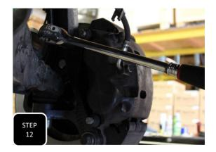
**Step 12** Attach the brake caliper to the spindle using the factory bolts and torque to 80 ft/lbs.
