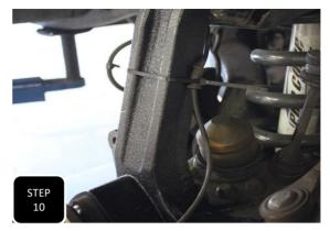
**Step 10** Install the ABS sensor using the factory allen bolt. Next, route the ABS line up the neck of the spindle and attach it to the neck of the spindle using the supplied zip tie.
