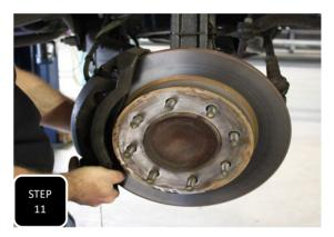
**Step 11** Slide the brake rotor onto the wheel bearing. Next, loosely install the brake caliper so that it is supported while installing the new, extended brake line.
