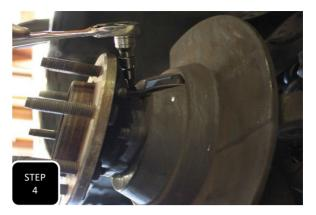
**Step 4** Remove the rotor and place it off to the side. Next, unbolt the ABS sensor and swing it safely out of the way so it does not get damaged during the install.
