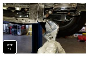
**Step 17** Some secondary skid plates will have a tab that will need to be bent to clear the diff mount. If your truck has this, bend it now.
