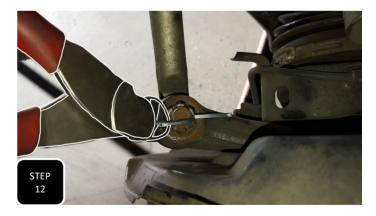
**Step 12** Re-attach the tie rod to the spindle and tighten. Once tight, re-install the factory cotter pin.
