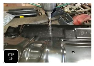
**Step 19** Once the diff drop spacers are tight, locate your primary skid plate. Using a 1/2" drill bit, enlarge the two forward most mounting holes.
