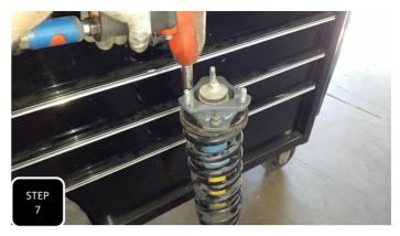
**Step 7** Remove the strut and then attach the strut spacer to the top of the strut using the factory nuts and tighten.
