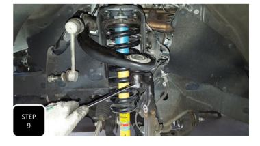
**Step 9** Place a floor jack under the lower control arm and jack up to compress the coil. Now re-attach the upper control arm to the spindle, tighten the castle nut, and re-install the factory clip.
