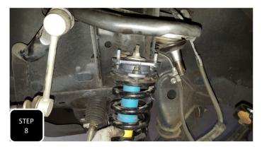
**Step 8** Re-install the strut assembly back into the truck and loosely attach the hardware at the top and bottom.
