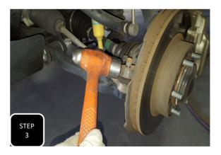
**Step 3** Loosen the tie rod nut, then break the tie rod loose by hitting the side of the steering arm with a hammer and separate. **NOTE: NEVER HIT THE TIE ROD ON THE THREADS.**
