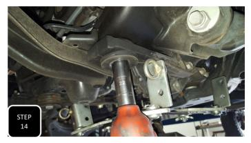
**Step 14** Place an adjustable jack under the front differential and remove the two front mounting bolts. **NOTE: THERE IS ONE MORE DIFF MOUNT TOWARDS THE BACK ON THE DRIVER'S SIDE THAT THE DIFF WILL PIVOT DOWNWARD ON.**
