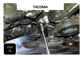
**Step 16** If your truck is equipped with a secondary skit plate directly below the differential, then remove the front two mounting bolts and for:
