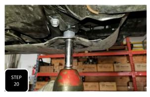
**Step 20** Re-install the skid plate using the provided 3/4" tall spacers along with the provided M8-1.25 x 40 bolts and washers near the diff and the facory bolts near the front bumper.
