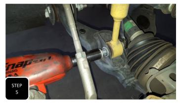
**Step 5** Loosen and remove the 3 nuts at the top of the strut and the single bolt at the bottom of the strut.
