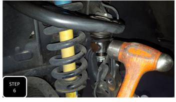
**Step 6** Remove the clip at the upper ball joint and then loosen the nut, but do not remove. Break the ball joint loose by hitting the side of the spindle with a hammer, the nut will catch the spindle, then separate. **NOTE: NEVER HIT THE BALL JOINT ON THE THREADS.**
