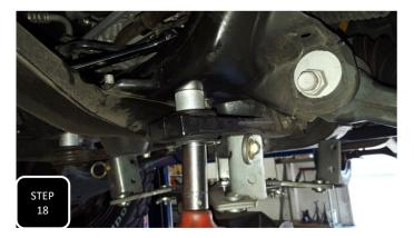
**Step 18** Lower the jack down and install the provided 1" tall spacers. Re-use the factory cup shaped washer at the bottom along with the provided 9/16" bolt, nut, and washer at the top. **NOTE: IF THE NYLOCK DOES NOT MAKE CONTACT WITH THE THREADS, OMIT THE WASHER.**
