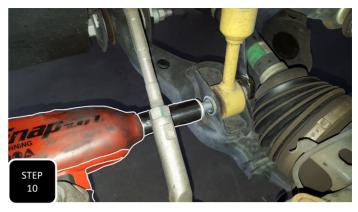
**Step 10** Tighten the provided nuts at the top of the strut and the factory bolt at the bottom.
