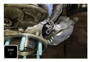
**Step 7** Unbolt the ABS sensor from the top of the hub, remove it, and then hang it up out of the way so that it does not get damaged during the install.
