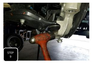
**Step 9** Loosen the nut at the lower ball joint, but do not fully remove it. Next, break the ball joint loose by hitting the side of the spindle, right at the ball joint, with a hammer. The nut will catch the spindle then you can fully remove the spindle. **NOTE: NEVER HIT THE BALL JOINT ON THE THREADS.**
