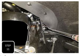
**Step 11** Unbolt both bolts attaching the upper control arm to the frame.
