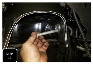
**Step 12** Remove the bolts and the control arm.
