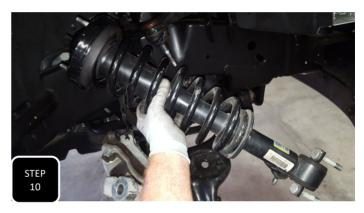
**Step 10** Remove the 3 mounting nuts at the top of the strut along with the 2 mounting nuts at the bottom. Next, with your knee or a pry bar, press down on the lower control arm so that the top of the strut separates from the coil bucket and then remove the strut.
