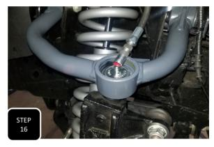
**Step 16** Pop the cap off of the top of the ball joint and add some grease to the grease fitting using a grease gun.
