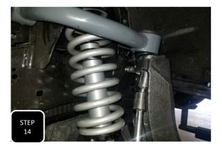
**Step 14** Reverse steps 1-10 to re-install the strut or coil over and your spindle. Next, attach the upper control arm to the spindle using the provided nut and tighten. **NOTE: 2021+ MODELS WILL SIT HIGHER THAN 2015-2020 MODELS. THE NUT WILL REACH THE END OF THE THREADS WITH NO EXTRA THREAD PAST.**
