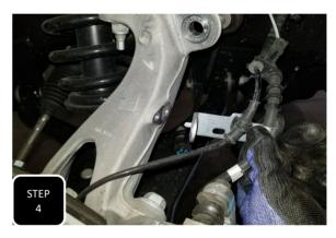
**Step 4** Unbolt the brake line guide bracket from the neck of the spindle and separate.
