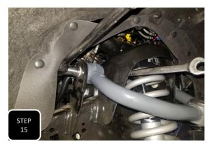
**Step 15** Repeat steps 1-14 on the other side. Once both sides are complete and the vehicle is back on the ground at ride height, then fully tighten the bolts attaching the upper control arm to the frame.
