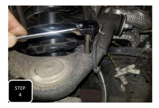
**Step 4** Open up the clamp attaching the ABS line to the upper control arm and then unbolt the bracket. This will allow for slack in the line while the spindle is separated from the upper control arm.
