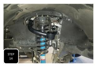
**Step 14** Re-attach the sway bar end link to the neck of the spindle and then re-attach both of the rubber skirts back into their original location.
