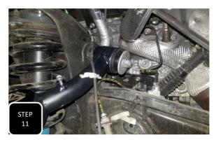
**Step 11** Locate the new control arm that is shaped like the one you just took off and loosely install it with the more rounded tube facing the front of the truck and the straighter tube facing the rear of the truck. **NOTE: DO NOT TIGHTEN THIS BOLT UNTIL THE TRUCK IS AT RIDE HEIGHT.**
