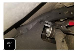
**Step 2** Gently pry to remove all of the clips attaching the rubber skirts on both sides of the control arm and remove the rubber skirts.
