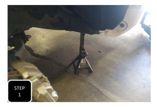
**Step 1** Jack up the front of the truck and support under the frame rail with a jack stand. Keep the floor jack under the lower control arm with pressure so that load is taken off of the upper control arm during the install.
