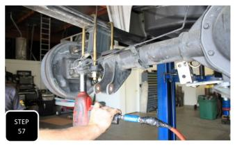
**Step 57** Loosely Install the provided U-bolts, from the top down and snug up the nuts under the factory spring plate. NOTE: DO NOT FULLY TIGHTEN THE U-BOLTS UNTIL BOTH REAR BLOCKS HAVE BEEN INSTALLED. ONCE BOTH ARE INSTALLED, TORQUE THE U-BOLTS TO 100 FT/LBS.
