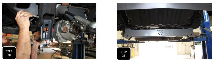
**Step 28** Loosely install the front subframe with the logo facing forward, using the factory hardware.
