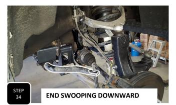
**Step 34** The ends of the sway bar originally swooped upward. The sway bar will now get re-installed with the ends swooping downward, the opposite of how they were. Use the factory bolts along with the provided nuts and washers to attach the sway bar to the drop down brackets and tighten.
