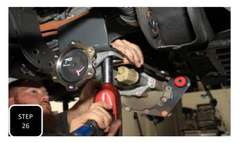
**Step 26** Place the differential back onto the adjustable jack and align it with the recently install diff drop brackets. Next, loosely attach the diff using the provided 1/2" bolts on the driver's side and 9/16" bolts on the passenger side. **NOTE: THE DIFF WILL GET FULLY TIGHTENED WHEN THE WHOLE FRONT END IS BACK TOGETHER.**
