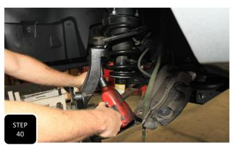
**Step 40** Install the steering knuckle assembly onto the the appropriate side that you are working on with the steering arm of the knuckle facing the front of the truck. Use the factory nuts at the upper and lower ball joints and tighten to factory specs. **NOTE: SLIDE THE AXLE INTO THE HUB BEFORE CONNECTING THE BALL JOINTS.**
