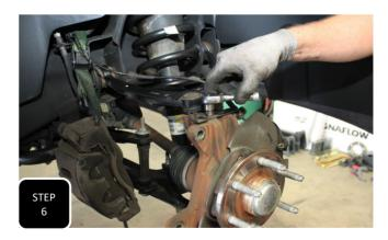
**Step 6** Unbolt the ABS sensor from the rotor and then the guide bracket from the top of the spindle. Support the ABS sensor out of the way so that it does not get damaged during the install.
