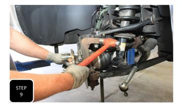
**Step 9** Loosen the upper ball joint nut, but do not remove. Hit the side of the spindle, right at the ball joint, with a hammer to break the ball joint loose. The nut will catch the spindle.
