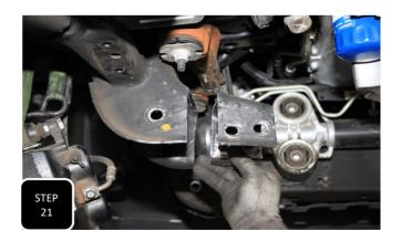
**Step 21** Working with the rearward lower control arm mount on the driver's side, mark a vertical line, 3 inches in from the inner edge where the original cross member was attached. Extend this mark straight up, across, and back down the front of the mount and then using a suitable cutting device, cut this section of the mount off.
