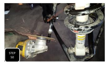
**Step 50** Mark a line 9/16" in from the threaded end of the inner tie rod and cut this section off. **NOTE: MAKE SURE TO CLEAN UP THE END SO THAT THE OUTER TIE ROD CAN THREAD BACK ON PROPERLY.**
