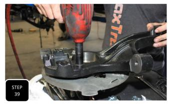
**Step 39** Place the factory hub assembly along with the factory dust shield onto the new steering knuckle and then flip the assembly over and attach the two together using the factory bolts and tighten.
