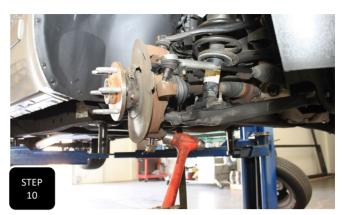
**Step 10** Loosen the lower ball joint nut, but do not remove. Next, hit the side of the spindle, right at the nut, with a hammer to break the ball joint loose. The nut will catch the spindle.
