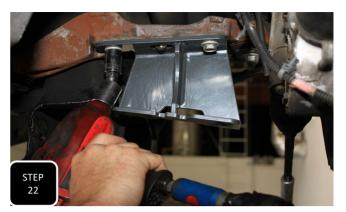
**Step 22** Locate the driver's side diff drop and install it to the factory mount using the factory hardware. The driver's side bracket has the tab that extendes past the bracket and an extra hole for the guide nipple in the factory mount. **NOTE: THE SHORT SIDE OF THE MOUNT WILL FACE THE REAR OF THE TRUCK.**
