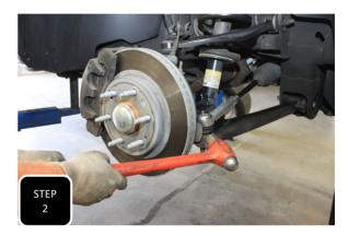
**Step 2** Loosen the tie rod at the spindle and break loose by hitting the side of the spindle, at the steering arm, with a hammer. **NOTE: NEVER HIT THE TIE ROD ON THE THREADS.**
