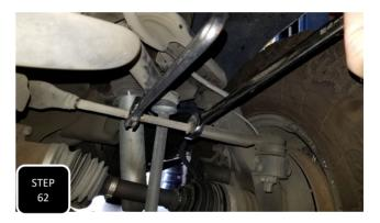
**Step 62** Install the new wheels and tires, then move the truck forward and back about 10 feet while moving the steering back and forth to settle the suspension. Next, adjust the vehicles toe alignment close to straight so that the vehicle is safe to drive to the alignment shop.
