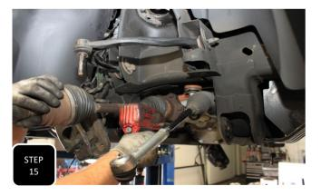
**Step 15** Unbolt all 6 bolts attaching the CV axle to the differential housing and remove the axle.
