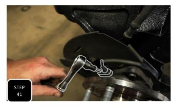
**Step 41** Unclip the ABS line from the frame, right next to where the brake line goes from soft to hard line. Next, use the extra slack gained to guide the ABS sensor down the steering knuckle and attach it to the wheel bearing using the factory bolt.
