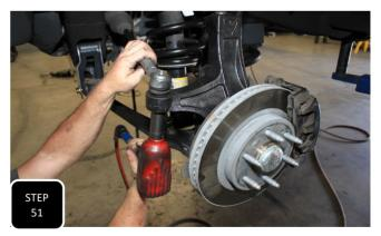
**Step 51** Once both ends are trimmed down, thread them back together and attach the tie rod to the steering knuckle using the factory nut.
