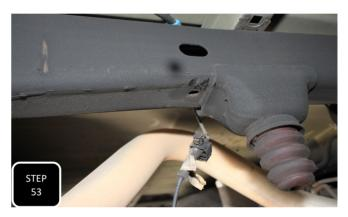
**Step 53** Apply some pressure to the diff with the adjustable jack and then remove both rear shocks. Next, Unclip both ABS sensor lines from the frame, just behind the bump stops. **NOTE: UNCLIPPING THE ABS LINES WILL ALLOW FOR EXTRA SLACK SO THE LINE DOES NOT GET DAMAGED DURING THE INSTALL.**
