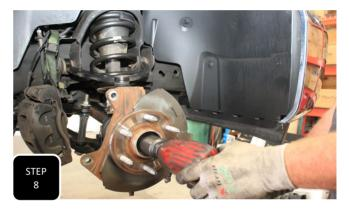
**Step 8** Pry off the dust cap at the end of the hub assembly and then remove the axle retainer nut.
