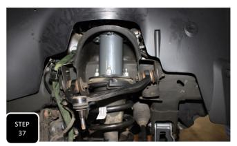
**Step 37** Fully tighten the upper mounting nuts and the lower mounting bolts for both struts.
