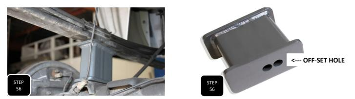
**Step 56** Install the new lift block. The lift block is angled and the short side must face the front of the truck. **NOTE: THE MAX TRAC LIFT BLOCK HAS TWO CENTER PIN HOLES. INSTALL THE CENTER PIN IN THE OFF-SET HOLE, WHICH WILL PUSH THE AXLE 1 INCH FORWARD AND MINIMIZE DRIVELINE PLUNGE.**
