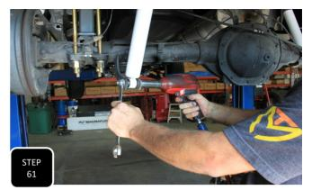
**Step 61** Install the new longer shocks using the factory hardware and tighten. **NOTE: MAX TRAC SHOCKS MUST BE MOUNTED WITH THE BODY AT THE AXLE AND THE SHAFT AT THE FRAME OR THEY WILL NOT WORK PROPERLY. FOX SHOCKS WILL MOUNT THE OPPOSITE, WITH THE BODY ON THE FRAME AND SHAFT AT THE AXLE.**
