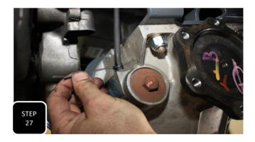
**Step 27** Plug the 4wd plug back into the diff and then stretch the breather hose down to the port on the diff and secure it using the provided zip tie.
