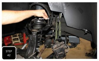
**Step 42** Using the provided loom clamps and factory 6 mm bolts, guide and attach the ABS line up the back side of the neck of the steering knuckle and to the upper control arm.
