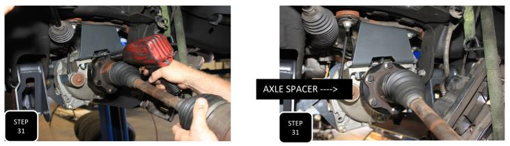
**Step 31** Using the provided M10 hardware, re-install both front axles with the aluminum spacers between the diff and axle.
