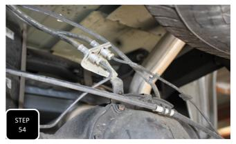
**Step 54** Using a pair of channel locks or a cresent wrench, bend the brakeline bracket on top of the diff so that the ends of the lines point up at the other end of the soft lines. **NOTE: BENDING THIS BRACKET CREATES MORE SLACK IN THE LINES.**
