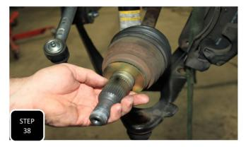
**Step 38** Slide the outer CV spacer onto the end of both axles with the chamfered I.D. side facing inward. The outer CV spacer is the 2 3/4" gold ring with a chamfered I.D. on one side.
