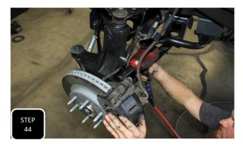
**Step 44** Unbolt the factory bracket that attaches the brakeline to the frame to gain extra slack in the line. Next, attach the brake caliper to the steering knuckle using the factory bolts and tighten.
