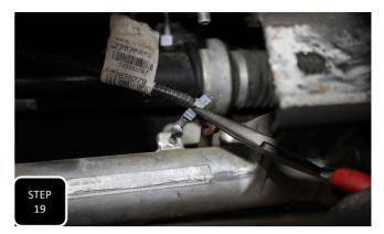
**Step 19** Unplug the wiring at the differential and separate the wire guide clip. Move the wiring up out of the way so that it does not get damaged during the install.
