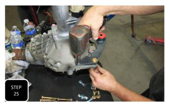
**Step 25** Remove the 4 bolts that the bracket aligns with and then install the bracket using the 4 provided M10-1.5 x 60 bolts and the 1 provided 7/16-14 x 3" bolt, nut, & washer then tighten. **NOTE: THE BRACKET WILL ONLY FIT ONE WAY AND ALWAYS TAKE CAUTION WHEN INSTALLING A STEEL BOLT INTO ALUMINUM THREADS.**
