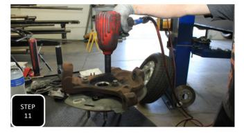
**Step 11** Remove the spindle and set it face down on the wheel studs. Next, remove all 3 bolts attaching the wheel bearing to the spindle and separate the two.
