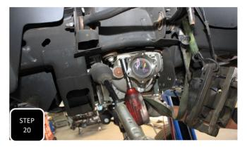
**Step 20** Support the differtial with an adjustable jack and then remove all 4 mounting bolts. Slowly lower the diff down making sure that there is nothing else attached to it that could get damaged.
