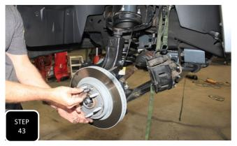
**Step 43** Install the rotor and secure the factory retainer screw.
