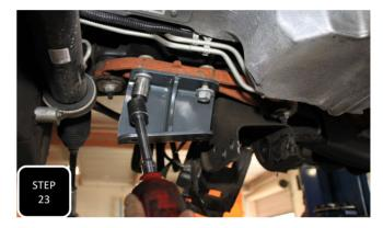
**Step 23** Locate and install the passenger side diff drop and attach it to the factory mount using the factory nuts, then tighten. **NOTE: THE SHORT SIDE OF THE MOUNT WILL FACE THE REAR OF THE TRUCK.**
