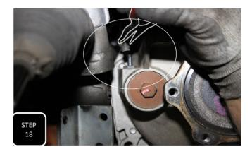
**Step 18** Remove all 4 bolts attaching the driveshaft to the front differential and then support the driveshaft up and out of the way. Next, detach the breather hose on the driver's side, top of the differential housing.
