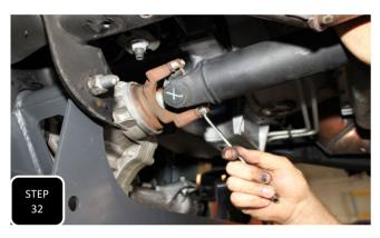
**Step 32** Attach the front driveshaft to the diff using the factory straps and bolts. **NOTE: IT IS NORMAL TO HAVE TO PULL THE DRIVESHAFT TO GET IT TO ATTACH TO THE YOKE.**
