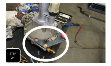
**Step 24** Take the differential and stand it upright on the driver's side axle flange. The breather port will leak a little if at a high point or a lot if at a low point. Place a vacuum cap over the breather for no fluid loss. Locate the provided dorsal fin diff bracket and line it up with the front side of the diff to see which bolts need to be removed.
