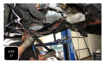
**Step 17** Unbolt the 4 bolts attaching the sway bar to the frame and remove the sway bar. **NOTE: TAKE NOTE THAT THE ENDS OF THE SWAY BAR SWOOP UPWARD. YOU WILL FLIP THIS OVER SO THEY SWOOP DOWNWARD WHEN THE SWAY BAR IS RE-INSTALLED.**
