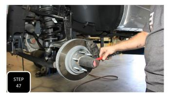
**Step 47** Install the axle retainer nut on both sides and torque to factory specs. Next, re-install the factory dust cap by tapping it into place with a mallet or dead blow hammer.
