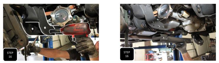
**Step 16** Unbolt the 4 bolts attaching the cross member to the rearward lower control arm mount and remove the cross member.
