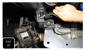
**Step 33** Install the sway bar drop down brackets using the supplied M10 bolts and washers. The open end of the bracket will face the inside of the truck and the bracket needs to swoop towards the rear of the truck.
