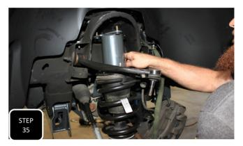
**Step 35** Locate the two struts and attach the strut spacer to the top using the factory nuts. Next, loosely install both sides using the provided nuts. **NOTE: THE SPACERS WILL ONLY FIT ONE WAY AND DO NOT FULLY TIGHTEN THE NUTS AT THE FRAME AT THIS TIME.**
