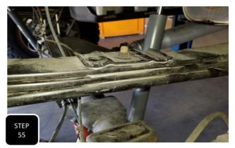
**Step 55** Working on one side at a time, remove the U-bolts and lower the axle down so that you have room to remove the factory lift block and insert the new one.
