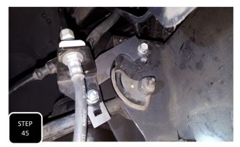
**Step 45** Locate the new brakeline mounting bracket and attach it to the side of the coil bucket using the factory brakeline bracket mounting bolt. Next, attach the factory brakeline bracket to the new brakeline bracket using the provided 8mm bolt, nut, and washers.
