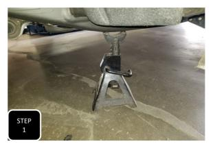
**Step 1** Jack up the front of the truck and support under the frame rails using jack stands.
