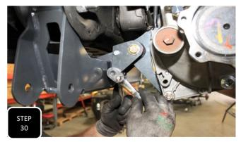
**Step 30** Attach the provided diff mounting ears to the back of the front subframe using the provided M8 hardware and then attach the diff to these ears using the provided 9/16" bolt, nut, and washers. Once all have been loosely installed, then fully tighten the diff ears and dorsal fin bolt. Next, fully tighten all of the diff bolts.
