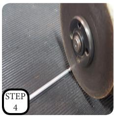
**STEP 4:** If you are installing 2" drop coils, then you will need to cut off the end of the new rod, right where the first groove ends, then install the rod ends and install back onto the truck.
