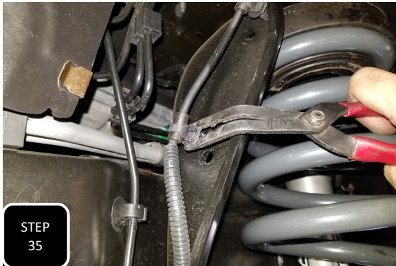
Step 35 Separate both ABS line guide clips from the front of the coil bucket on the frame and install the new ABS/brake line bracket using the provided M8 bolts, nuts, and washers. NOTE: THE DRIVER'S SIDE BRACKET IS THE LONGER OF THE TWO PROVIDED BRACKETS.
