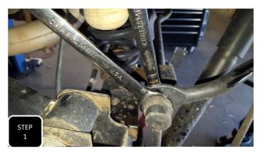
**Step 1** Unbolt both rear sway bar end links at both ends and remove. **NOTE: THE JOINT WILL WANT TO SPIN SO YOU WILL NEED A WRENCH ON BOTH SIDES OF THE MOUNTING PLATE.**
