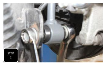
**Step 2** Attach the new enDlinks using the supplied 1/2" hardware at one end and the factory bolts at the other end. The endlinks will swoop inward at the top. **NOTE: SOME SWAY BAR HOLES WILL NEED TO BE OPENED UP SLIGHTLY WITH A** 1/2" DRILL BIT.
