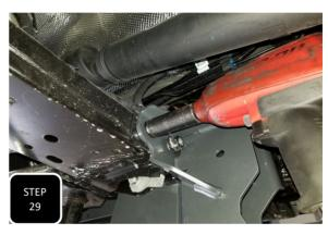
**Step 29** First snug up the U-bolt nuts, then the cross member bolts, and lastly the original radius arm bolt. Once all is snug and the bracket is up in place, go back and torque all bolts to factory specs. The U-bolt should get torqued to 100 ft/lbs.
