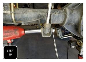
**Step 19** Install the new shocks and tighten. Max Trac shocks need to be installed with the shaft of the shock at the frame and the body at the axle. Fox shocks get installed opposite of that.
