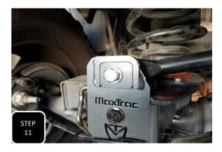
**Step 11** Use a rachet strap to pull the axle over and align the trac bar with the hole in the new bracket then loosely attach with the provided square plates and M14 bolt. The off-center hole will get installed with the bolt towards the driver's side for the 4" and 6" lift. Its only off-set to the pass side for the 8" lift. **NOTE: DO NOT TIGHTEN UNTIL THE TRUCK IS ON THE GROUND AT RIDE HEIGHT.**
