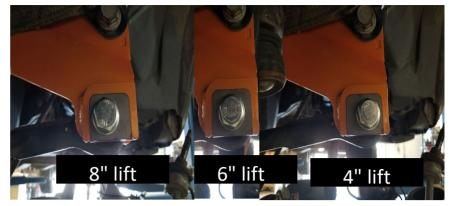
**Step 37** Slide the trac bar up into the new drop down bracket and loosely attach it using the provided M18 hardware and square plates. For the 4" lift, you will use the square plates with the off-center hole off-set to the driver's side. For the 6" lift, you will use the square plates with the centered hole. **NOTE: DO NOT FULLY TIGHTEN UNTIL THE TRUCK IS ON THE GROUND AT RIDE HEIGHT.**
