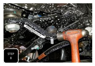
**Step 8** Remove the nut attaching the drag link to the pitman arm then brake the drag link loose by hitting the side of the pitman arm with a hammer, right at the joint, then separate. **NOTE: NEVER HIT THE THREADS OF THE ROD END.**
