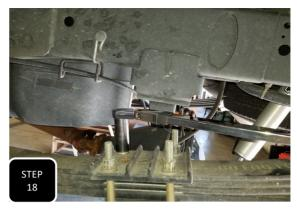
**Step 18** Install the provided U-bolts and loosely attach until both lift blocks have been installed. Next, torque the U-bolts to 100 ft/lbs.
