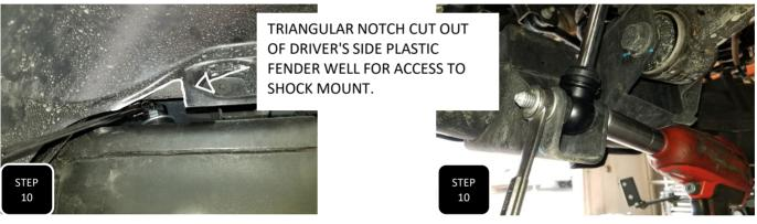
**Step 10** Install the new shocks and tighten down both ends. **NOTE: DO NOT OVER TIGHTEN THE TOP BUSHING OF THE SHOCK OR THE BUSHING WILL NOT BE ABLE TO FLEX AND COULD DAMAGE TO THE SHOCK.**
