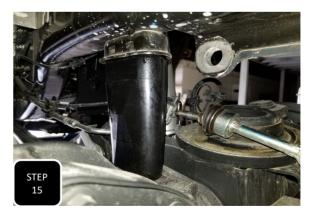
**Step 15** Locate the new, longer bump stops and spray the top of them with grease to make them easier to install. Next, line them up, one at a time, and using the jack under the axle as a press, jack the axle up until the bump stop presses into the cup all of the way.
