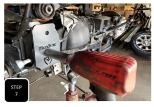
**Step 7** Loosely attach the trac bar bracket to the coil mount on the axle using the provided 3/8" hardware and then start the tightening process by tightening down the main trac bar bracket bolt to factory specs.
