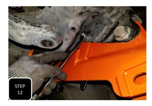
**Step 12** Loosely install the new trac bar bracket into the factory trac bar bracket using the factory bolt. Next, install the provided 7/16" bolt, nut and washer into the small tab mount further up the factory mount. **NOTE: DO NOT FULLY TIGHTEN EITHER BOLT AT THIS TIME.**
