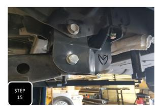
**Step 15** Loosely install the radius arm using the factory bolts at the axle and the provided M18 x 130 bolt at the bracket. NOTE: DO NOT FULLY TIGHTEN ANY OF THESE 3 BOLTS UNTIL THE TRUCK IS ON THE GROUND AT RIDE HEIGHT.
