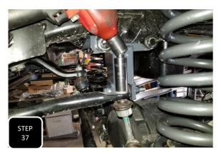
**Step 37** Attach the sway bar to the factory end links and tighten using the factory nuts.
