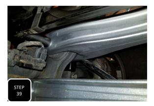
**Step 39** Re-install the wheels and tires then lower the truck to the ground. Once at ride height, tighten down the links to the axle. All 4 bolts will get torqued to 200 ft/lbs. **NOTE: IF INSTALLING THE RADIUS ARM KIT YOU WILL ALSO TIGHTEN THE BOLT AT THE FRAME BRACKET NOW, 6 BOLTS TOTAL FOR RADIUS ARM BRACKETS.**
