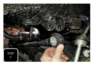
**Step 7** Remove the bolt attaching the trac bar to the bracket on the frame and separate. Allow the trac bar to rest on the axle.
