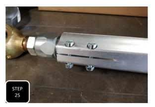
**Step 25** Get all 4 link arms in front of you with all of the Max Trac logos facing in the same direction and the two holed pinch seem facing up. Loosely install the provided M8 socket head bolts with the head of the bolt on the same side as the top of the Max Trac logo.
