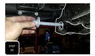
**Step 29** Loosely attach the links to the axle using the provided M18 bolts. After the first link is attached, you will want to remove one of the radius arm bolts, at the axle, on the other side so that the axle can be slightly rotated to attach the second link.
