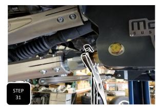
**Step 31** Tighten down both lower arm, M8 pinch bolts and then cinch down the two jam nuts on the rod ends. **REPEAT STEPS 20-31 ON THE OTHER SIDE.**
