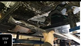
Step 19 Unbolt and remove the skid plate under the transfer case and set aside to be re-installed later.
