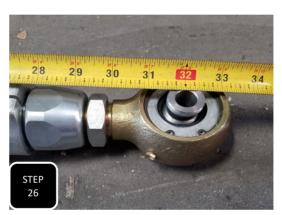
**Step 26** Adjust the upper links to 28.5" (the shorter link) and the lower links to 31 5/8" (the longer link). Now locate the links for the side that you are working on first. The driver's side links, when installed will have the Max Trac logo facing upright and the two pinch bolts facing outward when installed. **NOTE: THE ROD ENDS ARE NOT PRE-GREASED AND REQUIRE GREASE FOR PROPER FUNCTION.**
