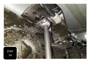
**Step 14** Loosely attach the provided  $1/2-13 \times 9$ " bolts, washers, and lock washers to the nut plate on top of the frame. Push the bracket up tight to the frame and torque the factory bolt to factory specs and the 1/2" bolts to 90 ft/lbs.
