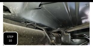
**Step 10** For the driver's side, you will need to create space between the wire harness on top of the frame and the module on the inside of the frame by prying the christmas tree retainer clips from the frame.
