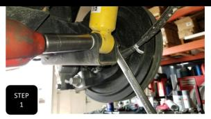
**Step 1** Jack up the rear of the truck and support under the frame with jack stands. Apply pressure to the rear diff with an adjustable jack and remove both rear shocks.
