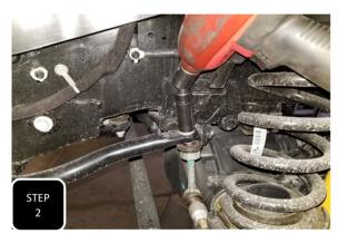
Step 2 Unbolt the sway bar from both end links and save the nut for re-installation.
