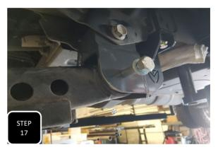
**Step 17** Loosely install the radius arm drop bracket using the factory bolt and push the bracket up tight against the frame, then tighten the U-bolt first. Next, torque the factory bolt to factory specs and the U-bolt to 100 ft/lbs.
