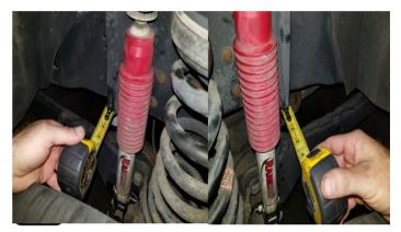
**Step 41** Loosen up the bolts for the clamps on the trac bar. Next. Find consistant measurement spots between each front tire and the frame, then adjust the trac bar until your measurements on both sides are equal then tighten down the clamp bolts.
