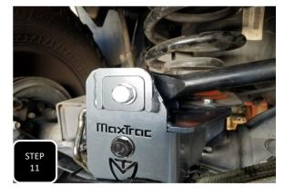
**Step 11** Use a rachet strap to pull the axle over and align the trac bar with the slotted hole and two square plates with the off-center hole. Off-set the bolt towards the passenger side of the truck for 8" lift. **NOTE: DO NOT TIGHTEN UNTIL THE TRUCK IS ON THE GROUND AT RIDE HEIGHT.**
