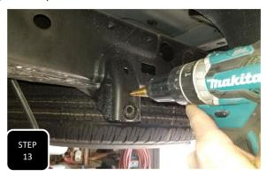
**Step 13** Loosely attach the sway bar drop down bracket to the factory bracket on the frame and mark the upper hole for drilling. Remove the bracket and drill a 7/16" hole at your mark. **NOTE: USING A STEP BIT WILL SPEED UP THE DRILLING.**
