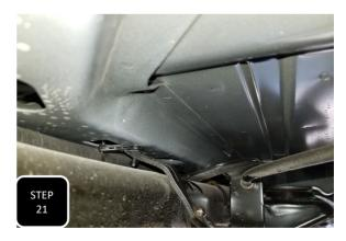
**Step 21** For the driver's side, you will need to create space between the wire harness on top of the frame and the module on the inside of the frame by prying the christmas tree retainer clips from the frame.
