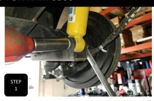
**Step 1** Jack up the rear of the truck and support under the frame with jack stands. Apply pressure to the rear diff with an adjustable jack and remove both rear shocks.
