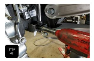
Step 42 Repeat step 38 on the other side and then tighten the top and bottom of both shocks.
