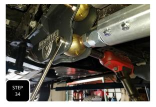
**Step 34** Tighten down the frame side bolts of the links completely and the axle side only hand tight. The axle side will get fully tightened when the truck is back on the ground at ride height.
