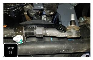
**Step 38** Loosen the clamp on the tie rod and adjust it out until you are able to rotate the rod end 180 degrees and then adjust it back in. **NOTE: THERE IS A PIN INSIDE THE TIE ROD THAT PREVENTS YOU FROM ROTATING THE END UNTIL YOU UNSCREW IT FAR ENOUGH TO DISENGAGE IT FROM THE PIN.**
