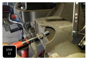
**Step 12** Unbolt the sensor rod ball from the mount on the axle and install the provided sensor brackets using the M6 bolt/washer at the original hole and the provided M8 bolt, nut & washer at the blank hole around the corner from the original bolt. **NOTE: USING A MAGNET WILL EASE THE PROCESS OF INSTALLING THE BOLT IN THE BLOCK ON THE AXLE.**
