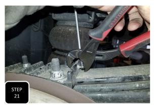
**Step 21** Re-attach the sensor rod to the spring plate using a set of channel locks to help pop the sock back onto the mounting ball then move to the other side and repeat steps 15-21 on the other side.
