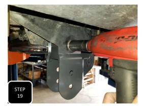
**Step 19** Push the bracket up tight against the frame and tighten the U-bolt first, then tighten the stock mounting bolt. Once tight, torque the factory bolt to factory specs and the U-bolt to 100 ft/lbs.
