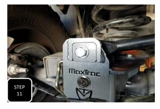
**Step 11** The plates with the off-center hole will get installed with the bolt towards the driver's side for the 4" and 6" lift. Its only off-set to the pass side for the 8" lift. **NOTE: DO NOT TIGHTEN UNTIL THE TRUCK IS ON THE GROUND AT RIDE HEIGHT.**
