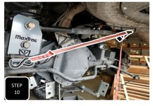
**Step 10** Use a rachet strap to pull the axle over and align the trac bar with the hole in the new bracket then loosely attach with the provided square plates and M14 bolt.
