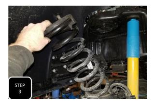
**Step 3** Move the jack to the driver's side of the axle and apply pressure. Then unbolt the drivers side shock from the axle and lower the axle so that you can remove the coil along with the rubber isolator.
