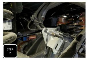
**Step 2** Using a cresent wrench or channel locks, grab the brake line bracket on the diff and bend it backwards to gain slack in the brake lines.
