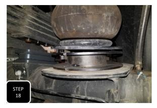
**Step 18** Install the lift block and the air bag spacer. The airbag spacer is off-set and when installed properly, the upper plate should off-set towards the rear of the truck with the ovalized holes facing the rear of the truck.
