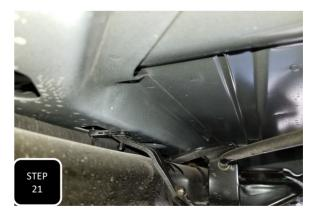
**Step 21** For the driver's side, you will need to create space between the wire harness on top of the frame and the module on the inside of the frame by prying the christmas tree retainer clips from the frame.
