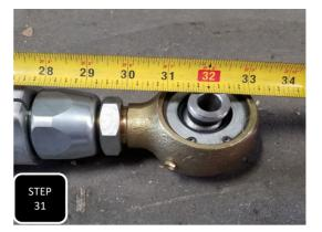
**Step 31** Adjust the upper links to 28.5" (the shorter link) and the lower links to 32" (the longer link). Now locate the links for the side that you are working on first. The driver's side links, when installed will have the Max Trac logo facing upright and the two pinch bolts facing outward when installed. **NOTE: THE ROD ENDS ARE NOT PRE-GREASED AND REQUIRE GREASE FOR PROPER FUNCTION.**
