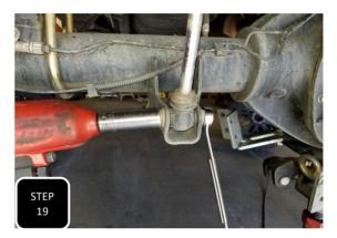
**Step 19** Install the new shocks and tighten. Max Trac shocks need to be installed with the shaft of the shock at the frame and the body at the axle. Fox shocks get installed opposite of that.
