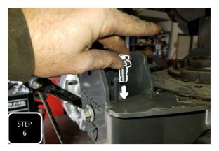
**Step 6** Slide the new trac bar bracket over the factory trac bar bracket on the axle and loosely install the factory bolt through the original trac bar mounting hole with the provided crush tube in the middle. Next, install one of the provided 3/8" bolts and washers through the inside, bottom of the bracket.
