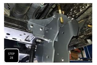
**Step 28** Locate the appropriate side 4link bracket so that when installed the Max Trac logo faces outward and the 2 holed side bracket faces inward. Loosely install the bracket using the factory radius arm bolt at the main hole, slide the two cross member bolts forward, and align the U-bolt with the top holes.
