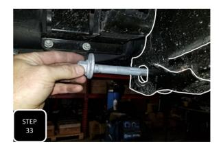
**Step 33** Loosely attach the links to the axle using the provided M18 bolts. after the first link is attached, you will want to remove one of the radius arm bolts, at the axle, on the other side so that the axle can be slightly rotated to attach the second link.
