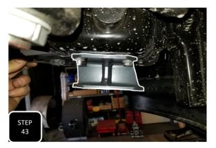
**Step 43** Locate and install the sway bar drop down brackets using the factory hardware. They are side specific and will get mounted with the open end facing the middle of the truck and side with the steeper angle facing the front of the truck.
