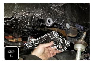
**Step 12** Remove the 5 bolts attaching the trac bar bracket to the frame and then remove the factory trac bar bracket.
