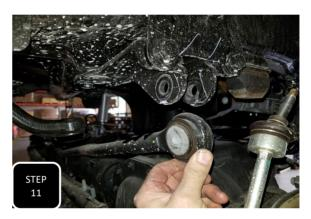
**Step 11** Remove the bolt attaching the trac bar to the bracket on the frame and separate. Allow the trac bar to rest on the axle.
