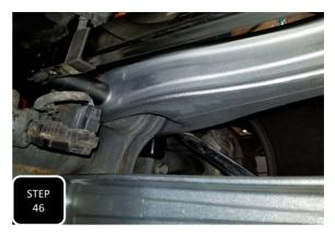
**Step 46** Re-install the wheels and tires then lower the truck to the ground. Once at ride height, tighten down the trac bar to the bracket and the links to the axle. All 5 bolts will get torqued to 200ft/lbs. **NOTE: IF INSTALLING THE RADIUS ARM KIT YOU WILL ALSO TIGHTEN THE BOLT AT THE FRAME BRACKET NOW.**
