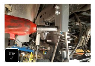
**Step 14** Attach the sway bar drop down bracket to the factory sway bar bracket using the provided 7/16" hardware and tighten. Next, attach the sway bar end link to the new bracket using the factory hardware and tighten. Repeat on other side.
