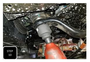
**Step 10** Apply a conservative amount of thread locker to the threads of the pitman arm nut then install the new, drop down pitman arm facing the same direction as the original one came off and torque to factory specs.
