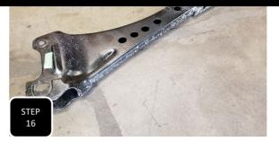
**Step 16** Working on one side at a time, remove the previously loosened radius arm bolts and then remove the radius arm.
