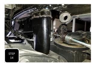
**Step 14** Locate the new, longer bump stops and spray the top of them with grease to make them easier to install. Next, line them up, one at a time, and using the jack under the axle as a press, jack the axle up until the bump stop presses into the cup all of the way.
