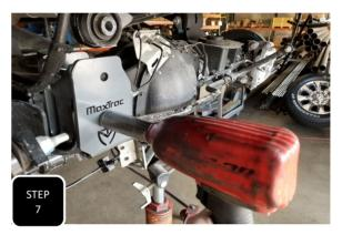
**Step 7** Loosely attach the trac bar bracket to the coil mount on the axle using the provided 3/8" hardware and then start the tightening process by tightening down the main trac bar bracket bolt to factory specs. **NOTE: IF THERE IS A GAP THEN USE THE PROVIDED SPACER BETWEEN THE COIL MOUNT AND BRACKET.**
