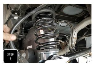
**Step 9** Set the new spacer onto the lower coil mount and then install the lower coil isolator onto the spacer. Next, reinstall both coils and jack up the axle until the coils are properly seated.
