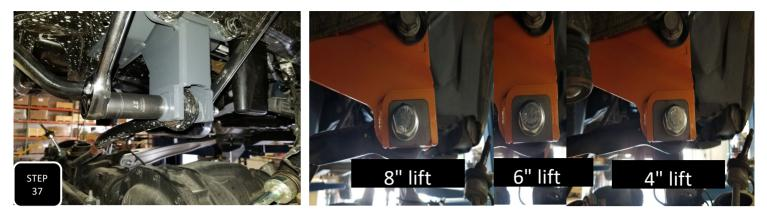
**Step 37** Slide the trac bar up into the new drop down bracket and loosely attach it using the provided M18 hardware and square plates. For the 4" lift, you will use the square plates with the off-center hole off-set to the driver's side. For the 6" lift, you will use the square plates with the centered hole. **NOTE: DO NOT FULLY TIGHTEN UNTIL THE TRUCK IS ON THE GROUND AT RIDE HEIGHT.**
