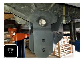
**Step 18** Slide the provided radius arm drop down bracket up into the factory mount and loosely attach using the factory bolt and the supplied U-bolt hardware.
