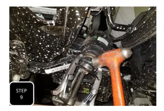
**Step 9** Remove the nut attaching the pitman arm to the steering box and then using a pitman arm puller or suitable 3 jaw puller, apply tension to the pitman arm and hit the side of the pitman arm with a hammer. After a few hits, tighten down the puller again and then repeat with the hammer until the arm separates.
