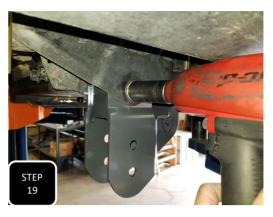
**Step 19** Push the bracket up tight against the frame and tighten the U-bolt first, then tighten the stock mounting bolt. Once tight, torque the factory bolt to factory specs and the U-bolt to 100 ft/lbs.
