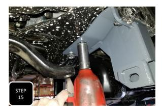
**Step 15** Install the new trac bar bracket using the original bolts along with the provided M14-2.0 nylock nuts. Make sure all the bolts are started in there threaded holes, then first, get all of the verticle bolts to a hand tight, then fully tighten the two horizontal bolts, and lastly tighten down the vertical bolts to factory spec.
