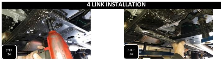
**Step 24** Unbolt and remove the skid plate under the transfer case and set aside to be re-installed later.
