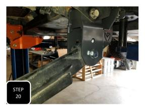
Install the radius arm into the: Upper hole for the 4" lift Lower hole for the 6" lift.
