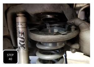
**Step 40** Move the jack to the driver's side of the axle and apply pressure. Remove the shock, lower the axle down, and first insert the isolator retainer into the rubber isolator. **NOTE: SPRAY WITH WD-40 FOR AN EASIER INSTALL.**
