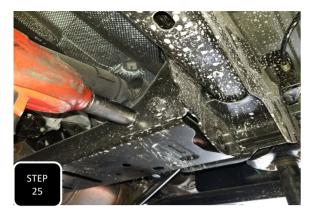
**Step 25** Remove the mounting nuts for the cross member just inside the radius arm bracket and push the bolts back so that the heads are not sticking out of the cross member.
