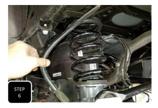
**Step 6** Set the new spacer onto the lower coil mount and then install the lower coil isolator onto the spacer. Next, reinstall both coils and jack up the axle until the coils are properly seated.
