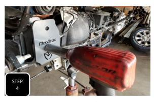
**Step 4** Loosely attach the trac bar bracket to the coil mount on the axle using the provided 3/8" hardware and then start the tightening process by tightening down the main trac bar bracket bolt to factory specs. **NOTE: IF THERE IS A GAP THEN USE THE PROVIDED SPACER BETWEEN THE COIL MOUNT AND THE BRACKET.**
