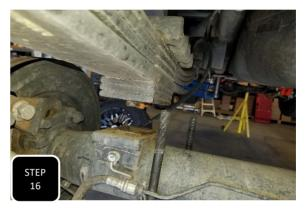
**Step 16** One side at a time, loosen both U-bolts, remove the U-bolts, and lower the axle to make room for the lift block. **NOTE: IT WILL HELP THE ALIGNMENT OF THE LIFT BLOCK TO SLIGHTLY LOOSEN THE U-BOLTS ON THE OTHER SIDE.**
