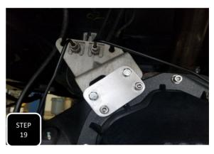
**Step 19** Remove the two bolts attaching the brake line bracket to the diff cover and loosely install the new brake line bracket using the factory bolts at the diff cover and provided M8 bolts at the brackets.
