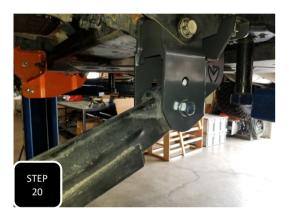
Install the radius arm into the: Upper hole for the 4" lift Lower hole for the 6" & 8" lift.
