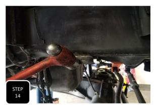
**Step 14** Using a suitable cuting device, cut the welds of the factory bump stop cup and then hit it with a hammer to break it loose. **NOTE: TRY NOT TO DAMAGE OR DISTORT THE CUP AS IT NEEDS TO BE RE-USED.**
