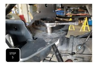
Step 5 Tighten up the two 3/8" bolts. NOTE: THE EASIEST WAY TO TIGHTEN DOWN THE BOTTOM 3/8" BOLT IS TO STICK A FLAT HEAD SCREW DRIVER DOWN INSIDE THE BRACKET AND WEDGE IT AGAINST THE HEAD OF THE BOLT WHILE TIGHTENING THE NUT WITH A RACTCHET.
