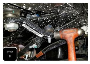
**Step 8** Remove the nut attaching the drag link to the pitman arm then break the drag link loose by hitting the side of the pitman arm with a hammer, right at the joint, then separate. **NOTE: NEVER HIT THE THREADS OF THE ROD END.**
