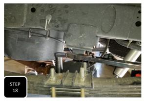
**Step 18** Snug down the U-bots on the first side, but do not fully tighten. Move to the next side, loosely install the lift block and new U-bolts, then when both sides are installed, tighten down the U-bolts and torque to 100 ft-lbs.
