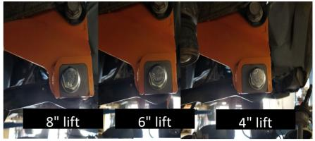
**Step 37** Slide the trac bar up into the new drop down bracket and loosely attach it using the provided M18 hardware and square plates with off-set hole. Install the plate so that the bolt is off-set to the passenger side of the truck. **NOTE: DO NOT FULLY TIGHTEN THIS BOLT UNTIL THE TRUCK IS ON THE GROUND AT RIDE HEIGHT.**
