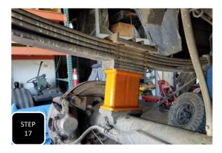
**Step 17** Install the new lift block. The block is flat so it can be installed either way. Align the center pins and jack up the axle to seat the block. **NOTE: IN SOME CASES, THE PLASTIC MIDDLE PIN MAY GET STUCK IN THE SPRING PERCH ON THE AXLE AND NEED TO BE PULLED OUT WITH PLIERS.**
