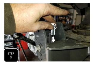
**Step 3** Slide the new trac bar bracket over the factory trac bar bracket on the axle and loosely install the factory bolt through the original trac bar mounting hole with the provided crush tube in the middle. Next, install one of the provided 3/8" bolts and washers through the inside, bottom of the bracket. **NOTE: DO NOT FULLY TIGHTEN EITHER OF THESE BOLTS AT THIS TIME.**
