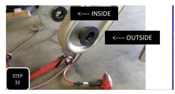
**Step 32** Loosely attach both links to the 4link bracket first using the provided 9/16" bolts and then install the provided machined, hat looking sleeves on the other end of the link with 1 hat inside the clevis and 1 hat on the outside.
