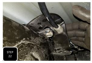
**Step 22** Insert the provided 9428RAB-2 nut plate on top of the frame, behind the E-brake bracket with the notched edge facing the front of the truck and the nut towards the outside of the frame facing downward. **NOTE: THIS E-BRAKE BRACKET IS ONLY ON 2021 AND NEWER TRUCKS.**
