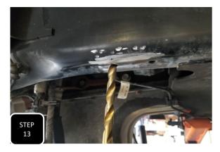
**Step 13** Drill out the holes in the frame using a 7/16" drill bit and then tap both holes using a 1/2-13 thead tapper.
