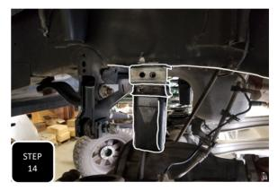
**Step 14** Attach the new bump stop bracket to the frame using the provided 1/2" bolts and then attach the factory bump stop cup to the new bracket using the provided 3/8" bolts, nuts, & washers. Next, spray some WD-40 onto the provided bump stop and pop it into the factory cup. **NOTE: JACKING UP THE AXLE AND USING IT TO PRESS THE BUMP STOP IN THE CUP WILL MAKE THIS MUCH EASIER.**
