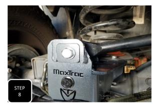
**Step 8** Use a rachet strap to pull the axle over and align the trac bar with the slotted hole and two square plates with the off-center hole. Off-set the bolt towards the passenger side of the truck for 8" lift kit with 5.5" rear lift spacers. **NOTE: DO NOT TIGHTEN UNTIL THE TRUCK IS ON THE GROUND AT RIDE HEIGHT.**
