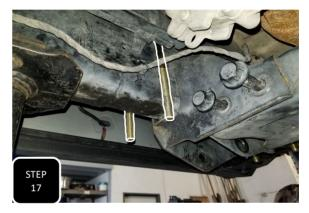
**Step 17** For the passenger side, slide the supplied U-bolt over the frame, just behind the cross member behind the factory radius arm bracket and allow it to hang vertically.
