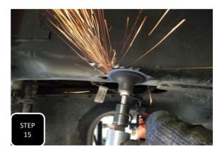
**Step 15** Once removed, clean up all sharp edges with a sander and then spray paint the frame to prevent rust.
