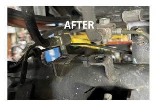
Some applications will require the brake lines to be unbolted from the axle and either stretch the hard lines or rotate the connection so that the end of the soft line points upward.
