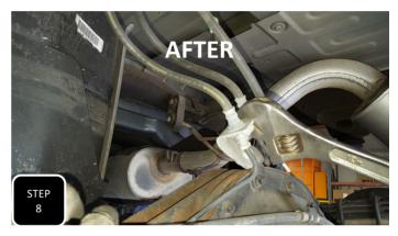
**Step 8** Always ensure that there is ample slack in brake lines, ABS lines, and any wires. You can usually gain slack in the factory brake lines by bending the mounting bracket upwards so that the end of the line is pointed directly at the other end.
