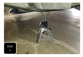
**Step 1** Jack up the rear of the truck and support under the frame rails with jack stands. Keep an adjustable jack under the differential for height adjustment.
