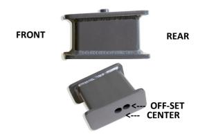
**Step 4** Loosely install the lift block with the short end facing the front of the truck and either with the factory center pin in the center hole or off-set hole. **NOTE: IF INSTALLING IN THE OFF-SET HOLE, YOU WILL WANT TO SLIGHTLY LOOSEN THE U-BOLTS ON THE OTHER SIDE TO ALLOW THE AXLE TO PIVOT.**
