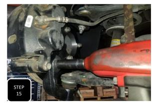
Step 15 Re-attach the brake caliper using the factory bolts and tighten down to factory specs.
