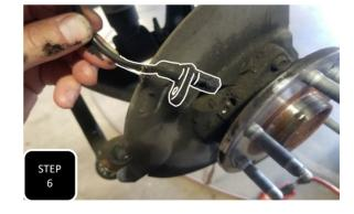
**Step 6** Unbolt the ABS sensor, separate, and hang up out of the way.
