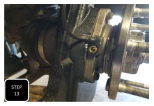
**Step 13** If your hub has an ABS sensor with the wire oriented 90 degrees out of the top of the sensor then you will need to clearance the side of your new spindle to make room for the wire. Using a suitable grinding devise, clearance out a small notch, enough to allow for the wire to clear and the sensor to fit down flush to the hub mounting surface.
