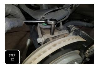
**Step 12** Re-attach the ABS sensor using the factory allen head bolt and tighten. Next, attach the ABS wire guide bracket to the top of the spindle using the factory 6mm bolt.
