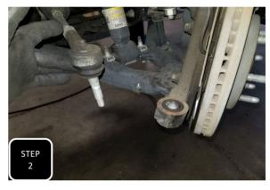
**Step 2** Unbolt the tie rod at the spindle and hit the side of the spindle, right at the rod end, with a hammer to break it loose and separate.
