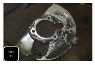
**Step 11** Attach the hub to the new spindle using the factory bolts and tighten to factory specs. **NOTE: THE FACTORY DUST SHIELD WILL "NOT" BE RE-INSTALLED.**
