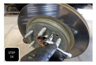
**Step 14** Slide the rotor over the wheel studs and secure it using the factory retainer bolt.
