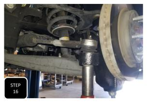
**Step 16** Attach the tie rod to the spindle using the factory nut and tighten to factory specs.
