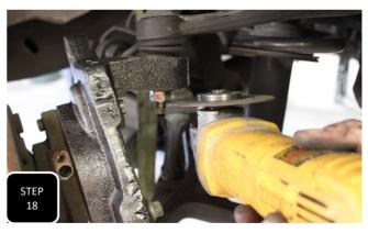
**Step 18** 4wd models will need to cut off the excess threads of the upper ball joint to clear the dust boot of the front axle.
