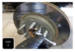
**Step 5** Unbolt the rotor retainer bolt and remove the rotor.
