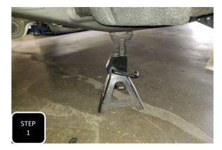
**Step 1** Jack up the front of the vehicle and support under the frame with jack stands.
