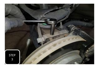
**Step 3** Unbolt the ABS wire guide from the top of the spindle and save for re-installation.
