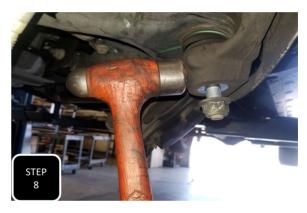
**Step 8** Brake each ball joint loose by hitting the side of the spindle with a hammer, right at the ball joint. The nut will catch the spindle, then remove the spindle.
