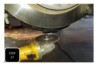
**Step 17** If you plan on running a 17" or 18" rim then you will need to replace the factory lower ball joint nut with the provided low profile nut and lock washer, then cut off the remainder of the lower ball joint threads. **NOTE: 16" RIMS WILL NOT WORK WITH THESE SPINDLES.**
