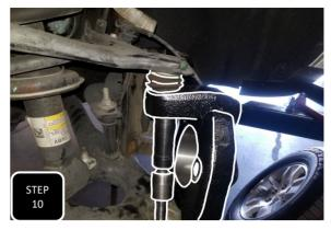
**Step 10** Locate the appropriate new spindle for the side you are working on and attach it to the truck using the factory ball joint nuts. Next, tighten to factory specs.
