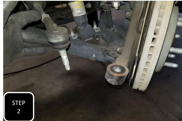
**Step 2** Unbolt the tie rod at the spindle and hit the side of the spindle, right at the rod end, with a hammer to break it loose and separate.
