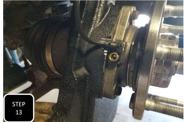
**Step 13** If your hub has an ABS sensor with the wire oriented 90 degrees out of the top of the sensor then you will need to clearance the side of your new spindle to make room for the wire. Using a suitable grinding devise, clearance out a small notch, enough to allow for the wire to clear and the sensor to fit down flush to the hub mounting surface.
