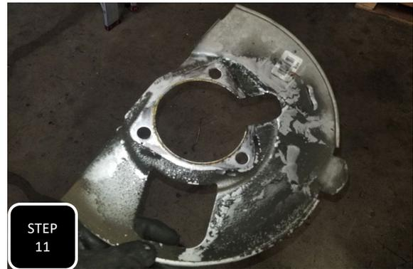
**Step 11** Attach the hub to the new spindle using the factory bolts and tighten to factory specs. **NOTE: THE FACTORY DUST SHIELD WILL "NOT" BE RE-INSTALLED.**
