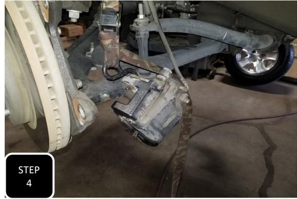
**Step 4** Unbolt the brake caliper and support out of the way. **NOTE: NEVER ALLOW THE BRAKE CALIPER TO HANG BY THE BRAKE LINE.**
