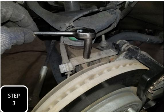
**Step 3** Unbolt the ABS wire guide from the top of the spindle and save for re-installation.
