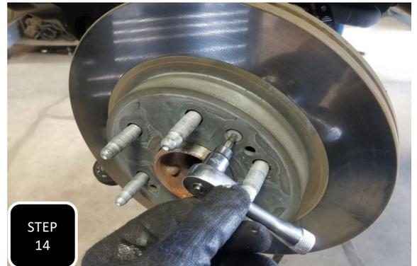
**Step 14** Slide the rotor over the wheel studs and secure it using the factory retainer bolt.
