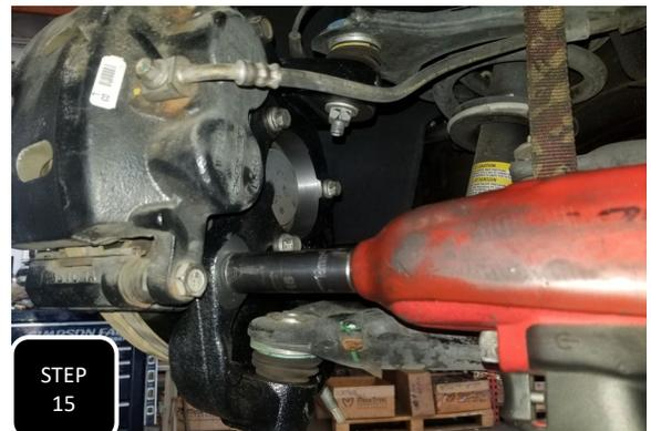
**Step 15** Re-attach the brake caliper using the factory bolts and tighten down to factory specs.
