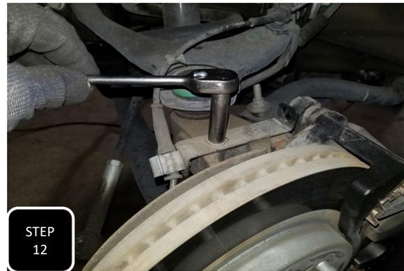
**Step 12** Re-attach the ABS sensor using the factory allen head bolt and tighten. Next, attach the ABS wire guide bracket to the top of the spindle using the factory 6mm bolt.
