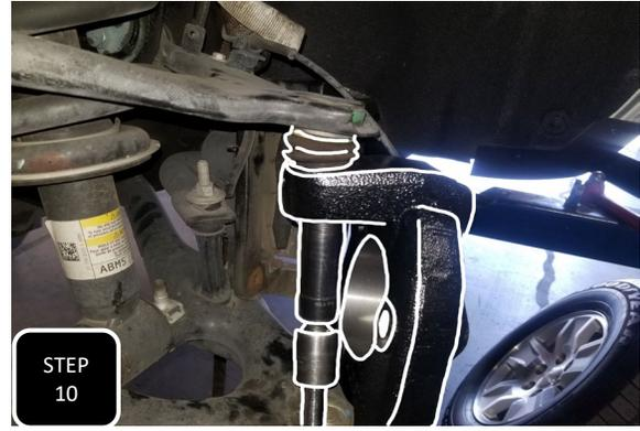
**Step 10** Locate the appropriate new spindle for the side you are working on and attach it to the truck using the factory ball joint nuts. Next, tighten to factory specs.
