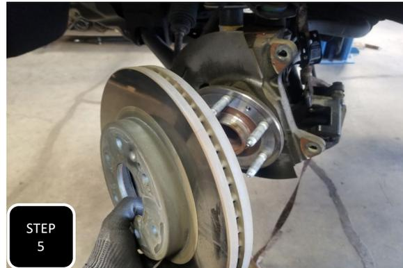
**Step 5** Unbolt the rotor retainer bolt and remove the rotor.
