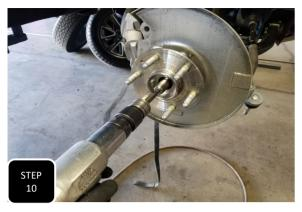
**Step 10** It is common for the axle to be a tight fit in the wheel bearing, so using a neumatic hammer to push the axle stub through the bearing may be necessary. **NOTE: NEVER DIRECTLY HIT THE AXLE WITH A HAMMER AS IT MAY DAMAGE THE THREADS.**
