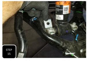
**Step 15** Unbolt the two bolts attaching the strut to the lower control arm and then insert the provided 1019AR-1 spacer plates between the strut's barpin and the control arm.
