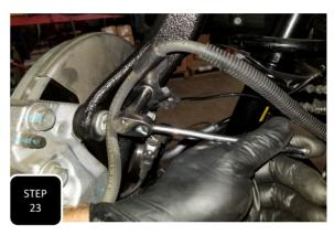
**Step 23** Attach the brake pad sensor wire to the neck of the spindle using the factory M6 bolt and then do the same with brake line bracket using the factory M6 bolt and tighten.
