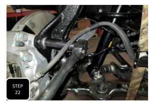
**Step 22** Attach the rotor by tightening the factory retainer bolt and then install the brake caliper using the factory bolts and tighten.
