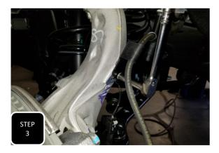
**Step 3** Unbolt the brake line guide bracket from the side of the neck of the spindle and separate.
