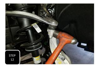
**Step 12** Loosen the nut attaching the upper ball joint to the spindle, but do not remove. Next, hit the side of the spindle, right at the ball joint, with a hammer, to break it loose and the nut will catch the spindle. **NOTE: NEVER HIT THE BALL JOINT ON THE THREADS.**
