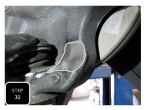
**Step 30** Using a 4.5" angle grinder with a flap disk or grind wheel, clearance this marked strike zone about 1/8" deep at the area of the contact point and smoothely transition your grind up and down.
