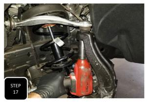
**Step 17** Install the new spindle using the factory upper and lower ball joint nuts and tighten. The upper balljoint will get torqued to 60 ft/lbs and the lower ball joint to 100 ft/lbs.
