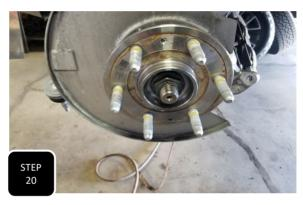
**Step 20** 4wd models will need to re-attach the axle to the wheel bearing using the factory nut and tighten to factory specs.
