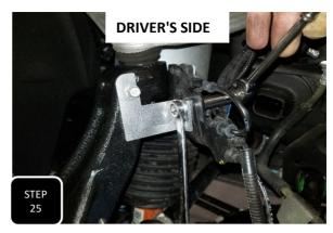
**Step 25** Models with air ride will attach the provided 1019AR-D bracket to the neck of the spindle using the factory M6 bolt and tighten. Next, attach the factory body position sensor to the bracket using the provided M6 bolt, nut & washers, then tighten.
