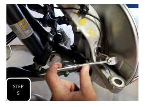
**Step 5** Unbolt the two ABS line brackets from the back of the neck of the spindle and the front of the spindle, then the ABS sensor itself. Next, separate the sensor and hang it safely out of the way.
