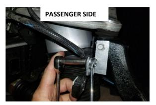
**Step 26** Attach the provided 1019AR-P bracket to the neck of the spindle using the factory M6 bolt and tighten. Next, attach the factory body position sensor to the bracket using the provided M6 bolt, nut & washers, then tighten.
