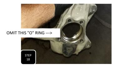
**Step 18** Install the wheel bearing along with the factory dust shield using the factory bolts and tighten to 40 ft/lbs. NOTE: THE SECONDARY "O" RING INSIDE THE HUB BORE OF THE FACTORY SPINDLE WILL NOT GET TRANSFERED TO THE NEW SPINDLES.
