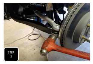
**Step 2** Unbolt the nut attaching the outer tie rod to the spindle and break loose by hitting the side of the spindle with a hammer, right at the tie rod. **NOTE: NEVER HIT THE TIE ROD ON THE THREADS.**
