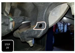
**Step 29** Start first by driving the truck and cycling the steering a few times to full turn so that a contact mark is left in the strike zone. Next, put the truck up in the air and mark about a 1.5" vertical area around the impact mark. This will be the area to clearance.
