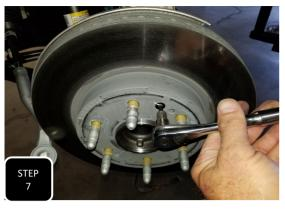
**Step 7** Unbolt the rotor retainer bolt and remove the rotor.
