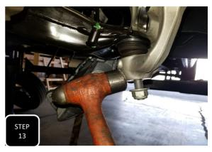
**Step 13** Loosen the nut attaching the lower ball joint to the spindle, but do not remove. Next, hit the side of the spindle, right at the ball joint, with a hammer, to break it loose and the nut will catch the spindle. Then remove the spindle. **NOTE: NEVER HIT THE BALL JOINT ON THE THREADS.**
