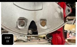
**Step 19** If your truck has a factory big brake kit then the factory dust shield will have an opening at the bottom and two studs sticking through the back side. The studs will need to be cut down flush on the back side of the dust shield or the will contact the face of the lowering spindle, pushing the dust shield outward, and causing the dust shield to rub against the rotor.
