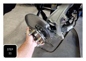
**Step 11** Separate the wheel bearing along with the dust sheild from the spindle and set aside for re-installation.
