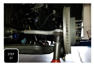
**Step 27** Lastly, attach the tie rod and tighten using the factory nut. Rotate the hub and make sure the dust shield is not rubbing the rotor, if it is then you may need to cut a little opening in the dust shield right at the tie rod. Once good, then repeat steps 1-20 on the other side.
