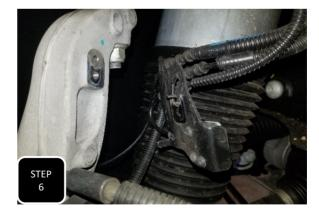
**Step 6** Air ride models will have a body position sensor attached to the upper ABS sensor bracket which gets removed just as step 5 shows. Unbolt this and the ABS sensor then move and hang safely out of the way.
