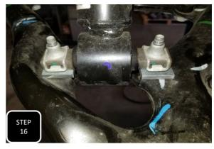
Step 16 Once both spacers are in place then re-install the factory bolts and tighten to 40 ft/lbs.
