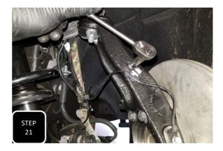
**Step 21** Attach the ABS sensor and the wire guide just above it to the new spindle using the factory M6 bolts.
