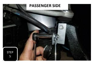
**Step 5** Attach the provided 1019AR-P bracket to the neck of the spindle using the factory M6 bolt and tighten. Next, attach the factory body position sensor to the bracket using the provided M6 bolt, nut & washers, then tighten.
