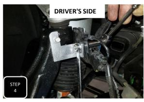
**Step 4** Models with air ride will attach the provided 1019AR-D bracket to the neck of the spindle using the factory M6 bolt and tighten. Next, attach the factory body position sensor to the bracket using the provided M6 bolt, nut & washers, then tighten. **NOTE: MODELS WITH MAGENERIDE WILL REQUIRE SEPARATING ONE SENSOR WIRE AND ROUTING IT A LITTLE BIT DIFERENTLY.**
