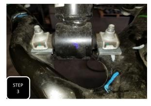
Step 3 Once both spacers are in place then re-install the factory bolts and tighten to 40 ft/lbs. NOTE: THE AXLES WILL STILL TOUCH THE LOWER AIR BAG MOUNT WHILE THE SUSPENSION IS AT FULL DROOP, BUT WILL NOT CONTACT DURING ANY NORMAL DRIVING.
