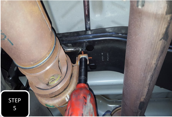
Step 5 Tighten the bolts down and torque them to 40 ft/lbs.
