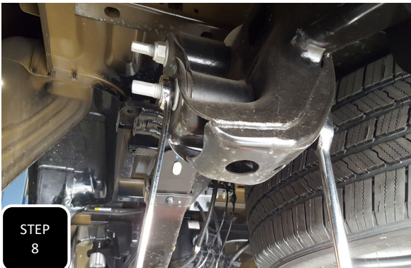
Step 8 Unbolt the shackle from the frame and then remove the bolt at the front of the spring and remove the leaf spring.
