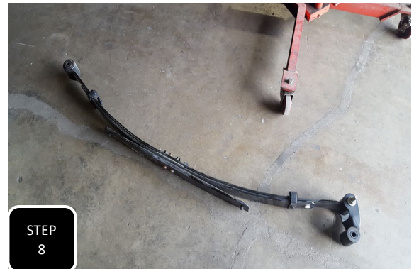
Step 8 Unbolt the shackle from the frame and then remove the bolt at the front of the spring and remove the leaf spring.
