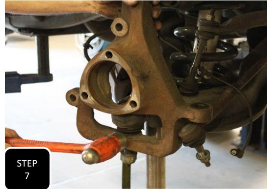
**Step 7** Loosen the lower ball joint nut, but do not remove. Next, break the ball joint loose by hitting the side of the spindle, right at the ball joint, with a hammer. The nut will catch the spindle then remove both the nut and the spindle.
