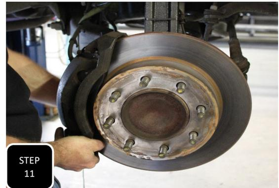
**Step 11** Slide the brake rotor onto the wheel bearing. Next, loosely install the brake caliper so that it is supported while installing the new, extended brake line.
