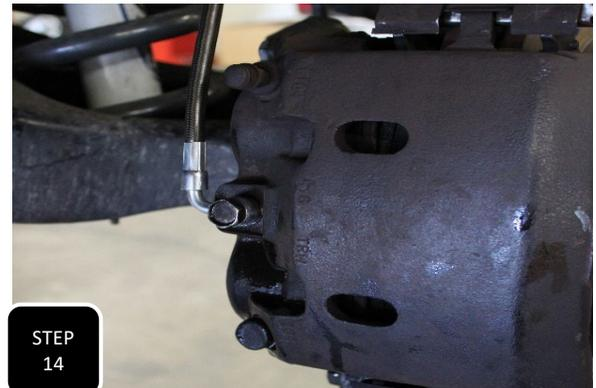
**Step 14** Attach the new, extended brake line to the hard line at the frame first and allow fluid to run through the line before attaching it to the brake caliper. Next, attach the brake line to the brake caliper using the factory banjo bolt and the provided copper crush washers. **NOTE: THE BRAKE LINE SHOULD BE POINTED STRAIGHT UP FROM THE CALIPER.**
