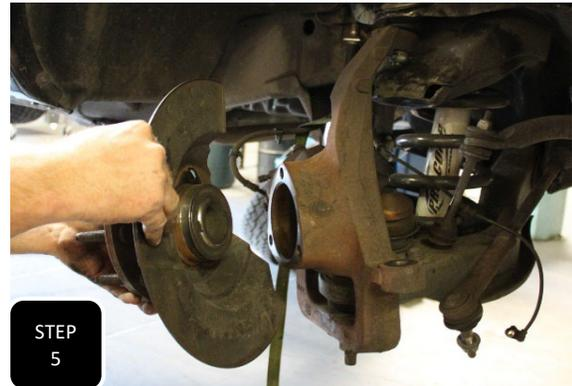
**Step 5** Unbolt the 3 wheel bearing mounting bolts and remove the hub assembly. **NOTE: THE FACTORY DUST SHIELD WILL NOT GET RE-INSTALLED.**
