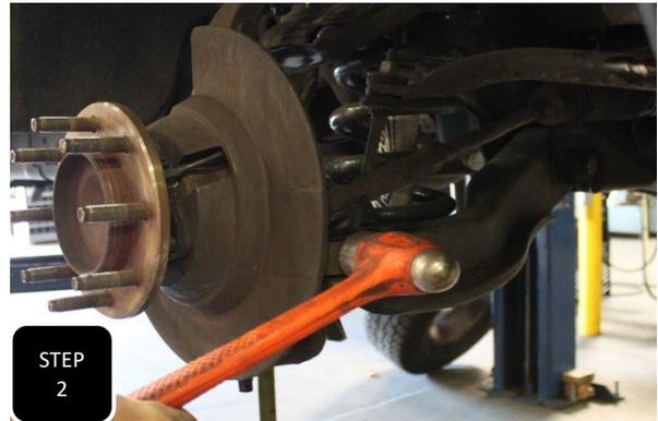
**Step 2** Unbolt the nut at the tie rod and break it loose by hitting the spindle with a hammer, right at the tie rod. **NOTE: NEVER HIT THE TIE ROD ON THE THREADS.**
