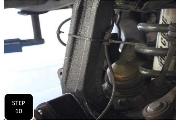
**Step 10** Install the ABS sensor using the factory allen bolt. Next, route the ABS line up the neck of the spindle and attach it to the neck of the spindle using the supplied zip tie.
