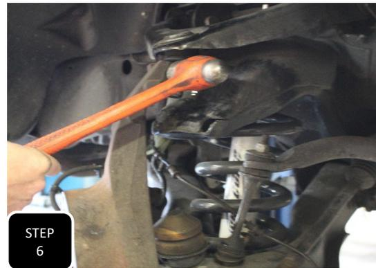
**Step 6** Loosen the upper ball joint nut, but do not remove. Next, break the ball joint loose by hitting the side of the spindle, right at the ball joint, with a hammer. The nut will catch the spindle then remove the nut. **NOTE: NEVER HIT THE BALL JOINT ON THE THREADS.**
