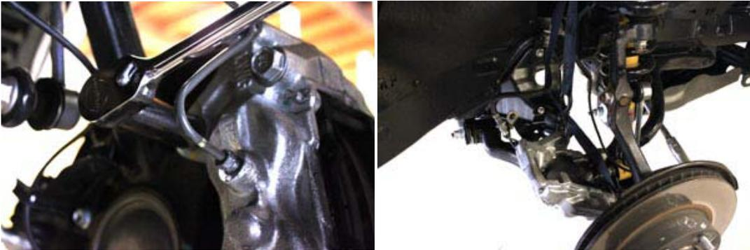
4. Remove brake rotor.
