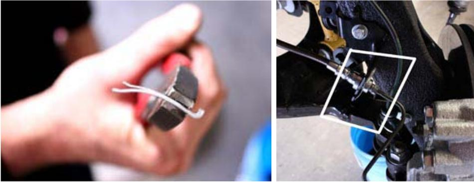
21. Remove the ABS line from behind the shock tower. Use supplied adell clamp to guide line across the Upper Control Arm, do the same with the clamps on the spindle using supplied bolts.
