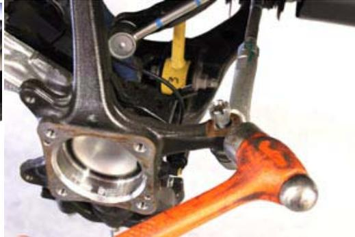
9. Remove the ABS Sensor, then upper ball joint nut.
