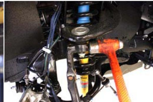
11. Guide ABS line down between the new spindle and lower ball joint/ steering stop plate. Slide lower ball joint into the double shear mount & attach upper ball joint to new spindle, tightening nut on ball joint, align cotter pin hole & install OEM cotter pin.
