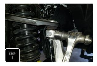
Step 6 Remove the retainer clip from the upper ball joint nut and then loosen, but do not remove the nut. Next, hit the side of the spindle, right at the upper ball joint, with a hammer to break the ball joint loose. The nut will catch the spindle then separate and allow the spindle to swing down. **NOTE: BE CAUTIOUS NOT TO DAMAGE THE BRAKE LINE OR ABS LINE.**
