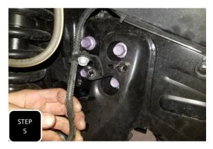
**Step 5** Unbolt the brake line guide bracket from the frame and separate. **NOTE: THIS WILL ALLOW FOR MORE SLACK IN THE LINE DURING THE INSTALL.**
