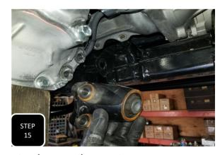
**Step 15** Loosen up all 3 bolts for the driver's side, front diff mount and remove the mount.
