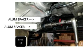
**Step 17** Lower the diff about 1 inch and then loosely install the new drive side diff mount using the provided M14 bolts and 1" aluminum spacers between the mount and diff. You will re-use the factory bolt and nut at the frame.
