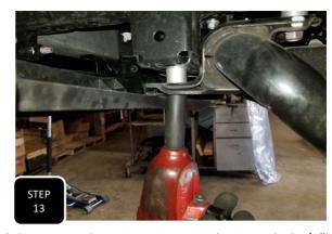
**Step 13** Loosen all 4 sway bar mounting bolts at the frame and then one side at a time, insert the provided 3/4" spacers and install them using the provided M12-1.25 x 60 bolts and washers. Once both sides have been installed, torque the bolts to 60 ft/lbs. **NOTE: THE SWAY BAR END LINKS WON'T GET INSTALLED UNTIL THE TRUCK IS BACK ON THE GROUND AT RIDE HEIGHT. REPEAT STEPS 3-13 ON THE OTHER SIDE.**
