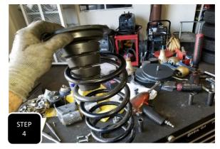
**Step 4** Lower the axle and remove both coil springs along with the bumpstop on top of the coils.
