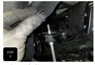
**Step 3** Unbolt both sway bar end links from the frame and remove the upper bushing.
