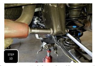
**Step 10** Once the truck is back on the ground at ride height, then you can re-attach the trac bar with more ease. You can use a ratchet strap from the frame to the axle, to align the bolt hole, if you are having trouble getting the upper bolt back in. Next, torque both bolts to 100 ft/lbs.
