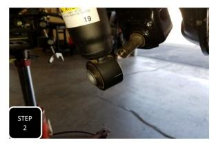
**Step 2** Apply some pressure to the differential with the jack and then unbolt both rear shocks at the axle and separate.
