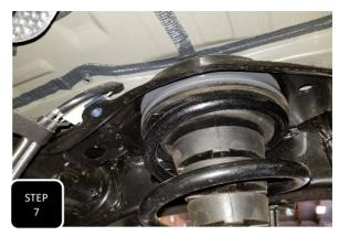
**Step 7** Lower the axle enough to install the coil with the spacer. Ensure that they properly seat top and bottom. **NOTE:** MAKE SURE THE BRAKE LINES AND ABS LINES HAVE PLENTY OF SLACK AND DO NOT GET STRETCHED OUT.
