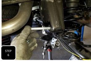
Step 6 Loosen both trac bar bolts and remove the upper bolt. NOTE: THIS WILL ALLOW FOR YOU TO LOWER THE AXLE MORE AND MAKE FOR AN EASIER INSTALL WITH THE ADDED HEIGHT OF THE SPACER.
