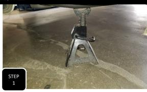
**Step 1** Jack up the rear of the truck and support under the frame rails with jack stands. Keep an adjustable jack under the differential for height adjustment.
