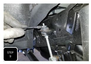
**Step 9** Re-install the upper sway bar bushings and tighten down. The bushings should have load applied to them, but not be crushed. "They need to move"
