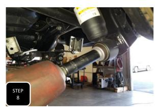
**Step 8** Jack up the axle and re-attach the shocks to the mount on the axle. Torque these bolts to 40 ft/lbs.
