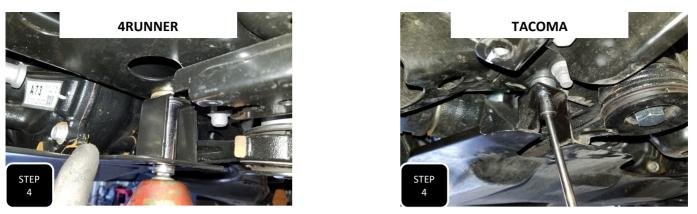
**Step 4** If your truck is equipped with a secondary skit plate directly below the differential, then remove the front two mounting bolts and for:
