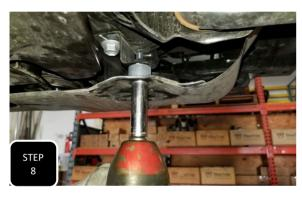
**Step 8** Re-install the skid plate using the provided 3/4" tall spacers along with the provided M8-1.25 x 40 bolts and washers near the diff and the facory bolts near the front bumper.
