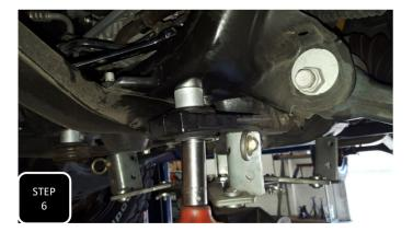
**Step 6** Lower the jack down and install the provided 1" tall spacers. Re-use the factory cup shaped washer at the bottom along with the provided 9/16" bolt, nut, and washer at the top. **NOTE: IF THE NYLOCK DOES NOT MAKE CONTACT WITH THE THREADS, OMIT THE WASHER.**
