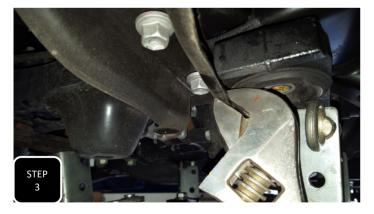
**Step 3** For models with stamped steel supports, bend down the lip of the sub frame support to make way for the diff mount in its new, lower position.
