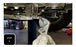
**Step 5** Some secondary skid plates will have a tab that will need to be bent to clear the diff mount. If your truck has this, bend it now.
