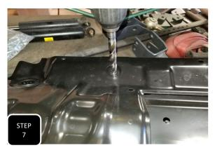
**Step 7** Once the diff drop spacers are tight, locate your primary skid plate. Using a 1/2" drill bit, enlarge the two forward most mounting holes.
