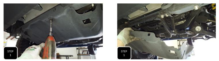
**Step 1** Unbolt all 4 bolts holding the primary skid plate on and remove the skid plate.
