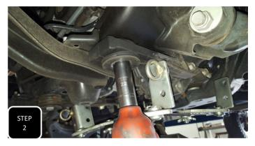
**Step 2** Place an adjustable jack under the front differential and remove the two front mounting bolts. **NOTE: THERE IS ONE MORE DIFF MOUNT TOWARDS THE BACK ON THE DRIVER'S SIDE THAT THE DIFF WILL PIVOT DOWNWARD ON.**
