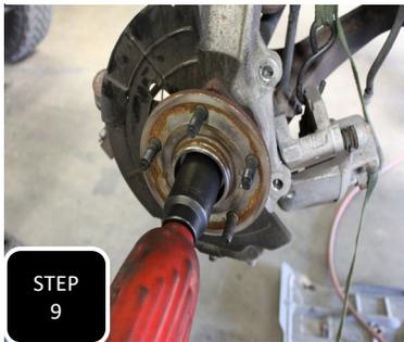
**Step 9** Remove the nut attaching the axle to the wheel bearing and then remove the ball joint nuts and the spindle.
