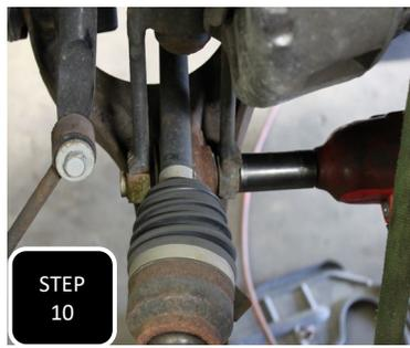
**Step 10** Unbolt the lower strut mount from the lower control arm, push down the lower control arm, and pivot the axle to the outside of the strut.
