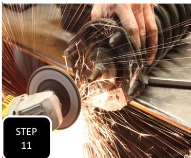
**Step 11** Remove the strut and grind down the factory studs to clear the bolt heads on the spacer. Once cleared, use the factory nuts to attach the spacer to the strut.
