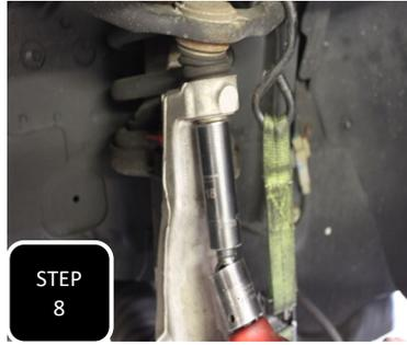
**Step 8** Loosen the upper and lower ball joint nut but do not remove. Break both ball joints loose by hitting the side of the spindle with a hammer, right at the ball joint. **NOTE: NEVER HIT THE BALL JOINTS ON THE THREADS.**
