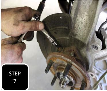
**Step 7** Unbolt the ABS sensor and then disconnect all clips attaching the ABS line to the neck of the spindle and support the sensor up out of the way.
