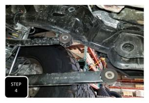
**Step 4** Working on the same side that you just removed the lower control arm, now loosen and remove the frame mounting bolt for the upper control arm and roll the axle forward.
