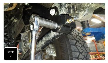
**Step 7** Loosely attach the lower control arm to the bracket using the provided M14 hardware. **NOTE: THE TIRE CAN BE ROLLED FORWARD OR BACKWARDS TO HELP ALIGN THE BOLT.**
