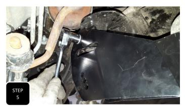
**Step 5** Loosely assemble the caster correction brackets using the provided 3/8" carriage bolts with the head of the carriage bolt on the inside of brackets. Locate the side that looks like it will fit the side you are working on and then install the brackets using the provided crush tubes and factory bolts. The outside ear will install inside the original mount and the inside ear will install on the outside of the original mount.
