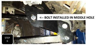
**Step 6** Loosely install the upper control arm to the axle and to the bracket. You can push or pull on the tire to help align the second bolt. There are 3 mounting holes for the upper control arm, use the upper hole if you have a 1.5-2" lift, the middle hole if you have a 2.5-3" lift and the lower hole if you have a 4-4.5" lift.
