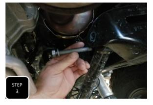
**Step 3** On one side only, loosen and remove the lower control arm bolt at the frame.
