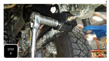
**Step 8** First tighten the two bolts that attach the bracket to the frame. Torque the top bolt to 70 ft/lbs and the bottom bolt to 100 ft/lbs. Next, only if you are installing with the truck on the ground torque the bolts attaching the control arms to the brackets to the same specs above. **NOTE: IF YOU ARE WORKING ON A LIFT, DO NOT FULLY TIGHTEN THE CONTROL ARM BUSHINGS UNTIL THE TRUCK IS BACK ON THE GROUND AT RIDE HEIGHT.**
