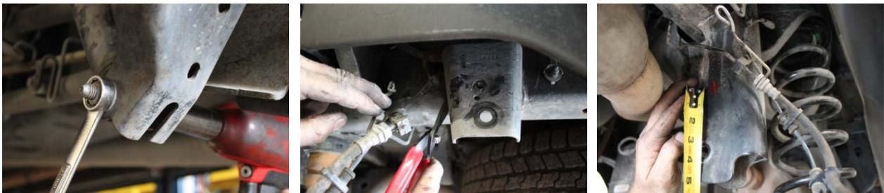
8. Drill a hole through your mark using a 7/16" drill bit. (The truck's exhaust may need to either be moved or removed to gain access with a drill)
