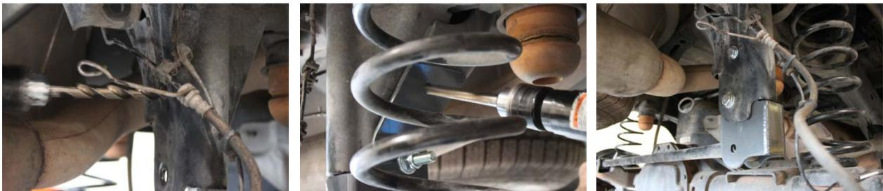
11. Install the new sway bar drop brackets using 1 provided bolt at the original sway bar mounting hole and the original brake line bolt at the threaded hole. Then install the brake line bracket at the proper side of the double hole using provided hardware.
